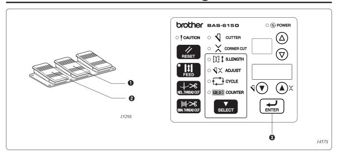
If the forward switch **①** is continued to be pressed at sewing, the clamp can be continued to operate in a specified interval.
