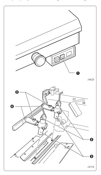
1. The marking light turns on when the power switch **1** is set to ON.
