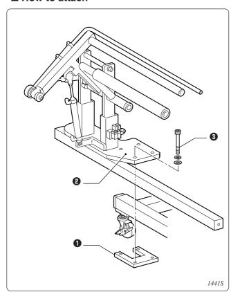
1. Set tap plate 1 at the bottom and the stacker base 2 at the top of the leg. Fix them with four bolts 3 respectively.
