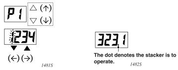
The program No., which is displayed to blink, has been selected. Press  $\Delta\nabla$  key to change the program No.(  $\mathcal{P}$ -( $\mathcal{P}$ -) is used when no setting is performed for the program.) Setting or releasing can be performed for the stacker operation at this step. Set the program No. you want to set or release to blink and press the "SELECT" key ③. When the stacker operation is set, a dot appears at the lower and right side of the program No.
