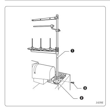
Put cotton stand 1 into bracket 2 and fix with screw 3.
