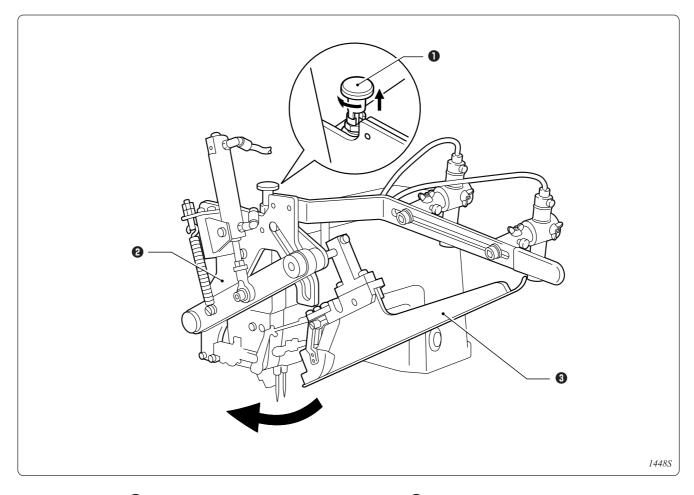
Pull up plunger 1 and lock it, and then open main plate 2.
