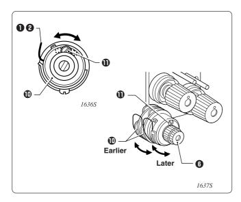
The standard operation timing for thread takeup spring L ① and thread take-up spring R ② is the middle position within the operating range of the thread take-up spring guide ①.
