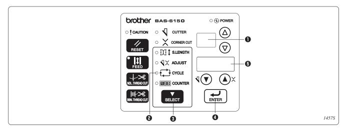
Five kinds of cycle program can be generated. Four programs can be set for each cycle program. The cycle program can be modified. Setting or releasing can be performed for the stacker operation in the cycle program.
