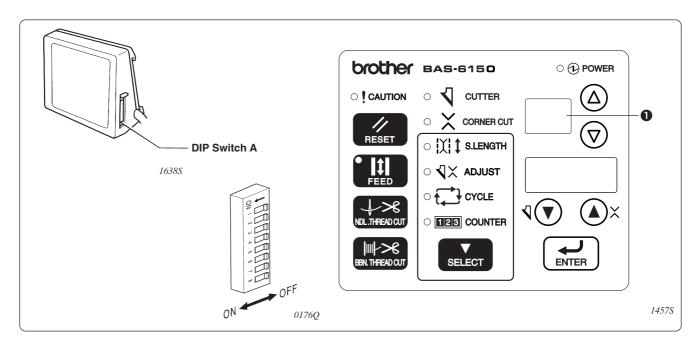
Turn off the power switch, and turn on the DIP-SW A8 on the operation panel. Program will be locked when the power switch is turned on.
