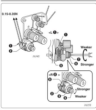
The standard tension for thread take-up spring L 1 and thread take-up spring R 2 is 0.15-0.35N for both springs.
