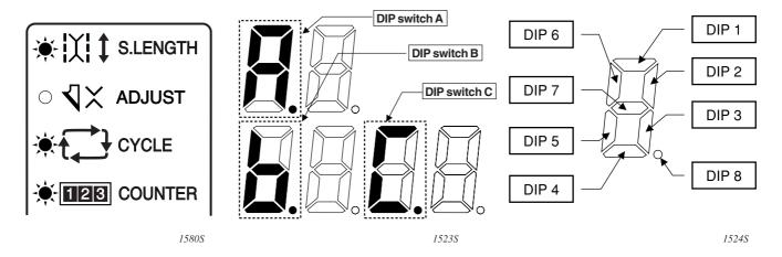
The corresponding segment lights on when the DIP switch is ON.
