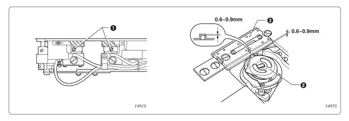
Loosen screw 1 and let the rotary hook 2 up and down so that the clearance between rotary hook 2 and needle plate 3 be 0.6 - 0.9mm.
