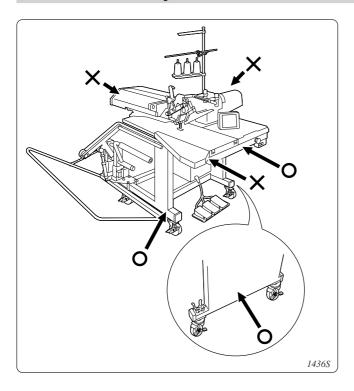
Lift up the main body (the frame) to carry the machine.
