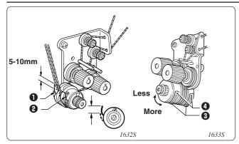
The standard operating range for thread takeup spring L ① and thread take-up spring R ② is 5-10mm for both springs.
