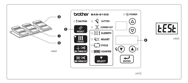
Operation of the switch can be performed for each step. In the test operation mode, the machine, center knife, and corner knife do not operate.
