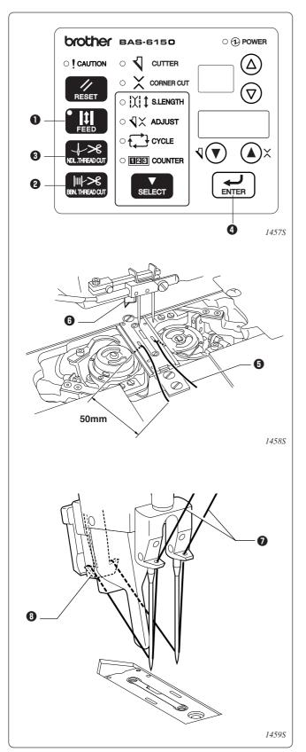
1. Press the "FEED" key 1 to move the carriage feed to the feed position.
