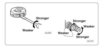
After the lower thread tension has been adjusted, adjust the upper thread tension.
