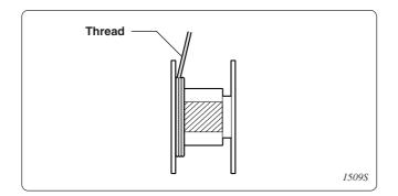
(Note) Be sure to wind the thread either right or left end of the groove. Winding from the center can not guarantee the precise detection of remaining amount of threads.
