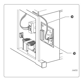
5. Connect bar stacker harness (1) to P20 on main circuit board (1) in the control box.
