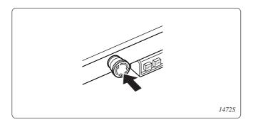
Machine operation can be stopped by pressing the emergency stop button. The emergency stop button is of push turn lock type.
