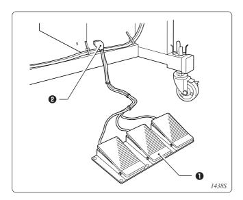
Plug connector **②** of 3-pedal foot switch **①** into the connector on the front side.
