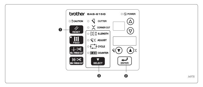
Initialization of the unit memory can be performed by pressing a certain key when the power supply switch is turned ON.
