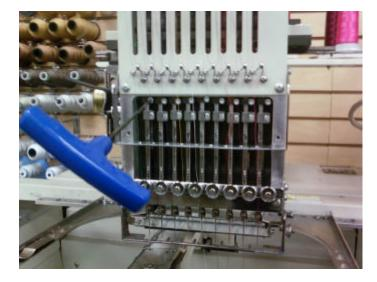
3. Loosen Top Dead Center Stopper screw with a 2.5mm hex wrench on all the needles.
