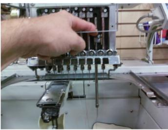
5. Push down on the Top Dead Center Stopper with one hand. <u>Do not</u> <u>release it until instructed to do so</u>. While holding the Top Dead Center Stopper down with one hand, use your other hand to pull down on the needle bar until the top of the needle bar is exposed as shown in the picture.
