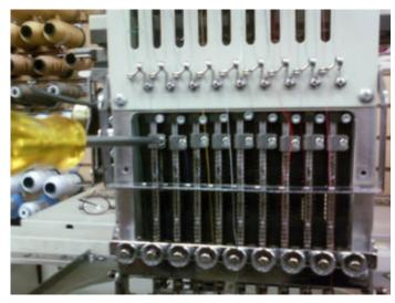
4. Loosen the Needle Bar Clamp screw on all the needles.
