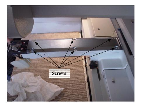
Once you have the cover removed you will be able to access the adjustment screws for the moving knife. Loosen the screws as indicated in the photo below and move the moving knife with your fingers until you get it 1 mm from the edge of the fixed knife. Re-tighten your adjustment screws and press the thread-trimming button on the machine and re-check the adjustment. You may have to do this more than once to achieve the correct position.
