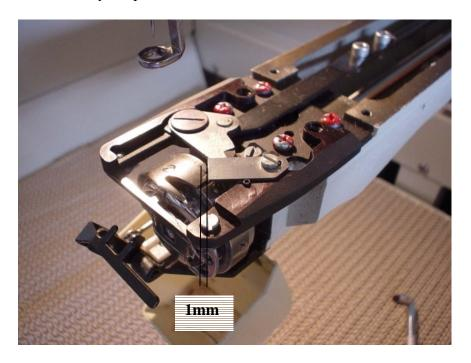
If you find the moving knife needs to be adjusted. You will need to remove the arm cover by removing the 6 screws as indicated in the photo below.
