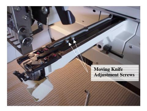
Re-install the arm cover and the needle plate and your finished.
