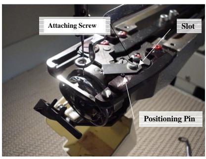
After you have checked and adjusted, if necessary, the fixed knife. Now we can check the moving knife. The tip of the moving knife should protrude past the edge of the fixed knife 1 mm as illustrated by the photo below.
