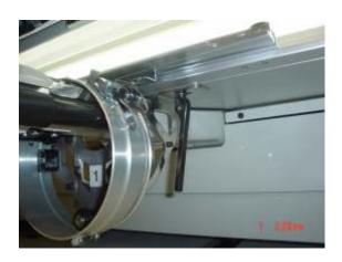
6. Flip mode switch on machine to CAP. Turn power ON.
