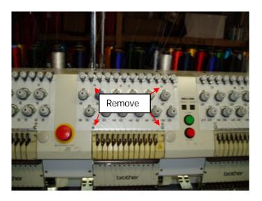
10. Remove the four hex screws securing the tension base. Remove tension base from the machine by disconnecting the harness at the back and the ground wire held on by a screw to the tension base mount.
