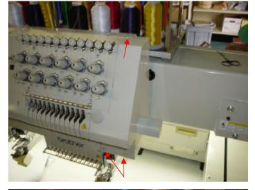
3. Remove the right end cover by removing the two lower screws and loosening the one upper screw.
