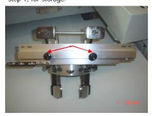
5. Install tubular arms. Flip mode switch on machine to FLATS. Turn power on.
