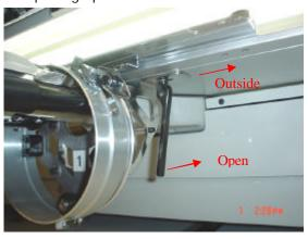
4. Remove the cap driver from the bed and fix the cap frame sash with the black thumbscrews, removed in step 1, for storage.
