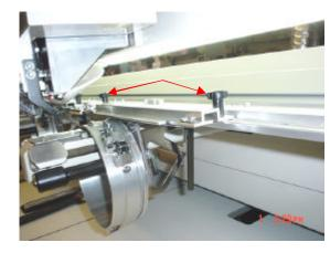
2. Hold up the cap frame sash and remove it from the positioning pins by moving slightly forward.
