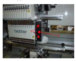
13. Grease the cam groove of the thread take-up driving cams.
