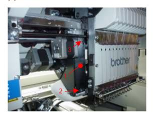
6. Unscrew the two adjusting bolts [4] and detach the jump part stepping motors [5].
