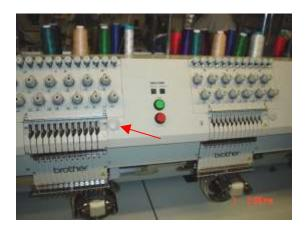
2. Wet the top of the felt pads with oil.
