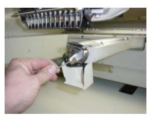
Insert bobbin cases in to rotary hooks. Make sure bobbin thread is not over 2 inches long. Close bobbin case covers.
