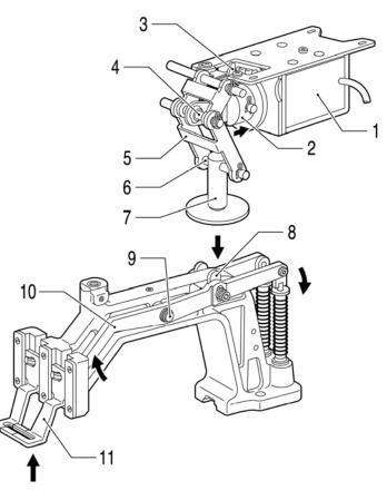
\* When the presser solenoid is turned off, the presser plate rises, and work clamps lower.
