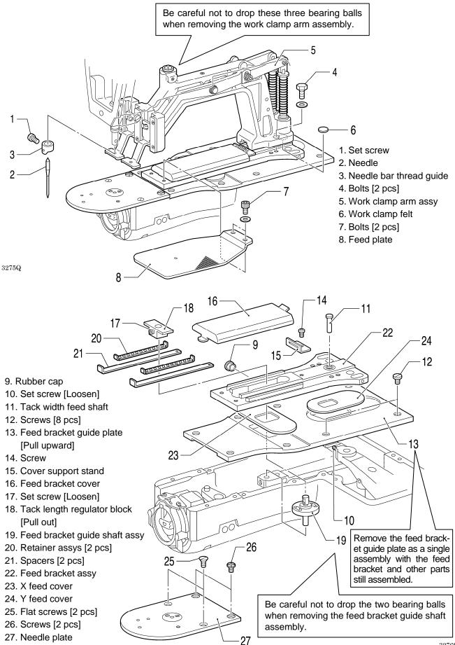
3 - 5 . Work clamp arm mechanism (KE-434B, 434C, 435B, 435C, 436B, 436C, 484C)
