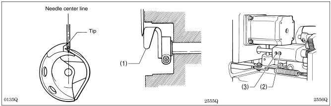
Turn the machine pulley to align the tip of the rotary hook with the needle center line. Then loosen the set screw (2) and turn the eccentric shaft (3) to adjust so that the driver needle guard (1) contacts the needle.
