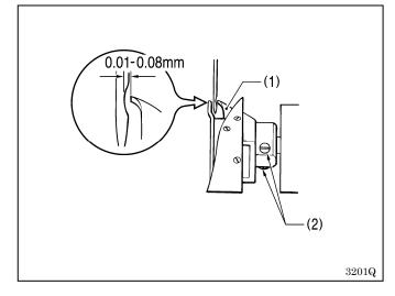
Turn the machine pulley to align the tip of the rotary hook (1) with the needle center line. Then loosen the set screw (2) to adjust so that the clearance between the needle and the rotary hook (1) is 0.01 - 0.08 mm.
