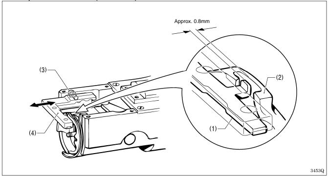
Loosen the screw (3) and move the hook stopper setting base (4) to adjust so that the tip of the bobbin case holder position bracket (1) is approximately 0.8 mm away from the needle drop surface.
