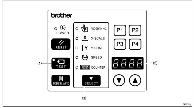
1. While pressing the TEST switch (1), turn on the power to the machine. Version number of each PROM can be confirmed in display (2).
