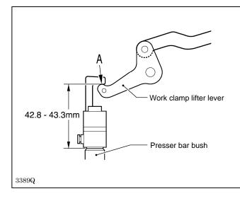
Install the air cylinder setting plate so that there is a distance of 42.8–43.3 mm between section A of the work clamp lifter lever and the top of the presser bar bush when section A is at its lowest point.
