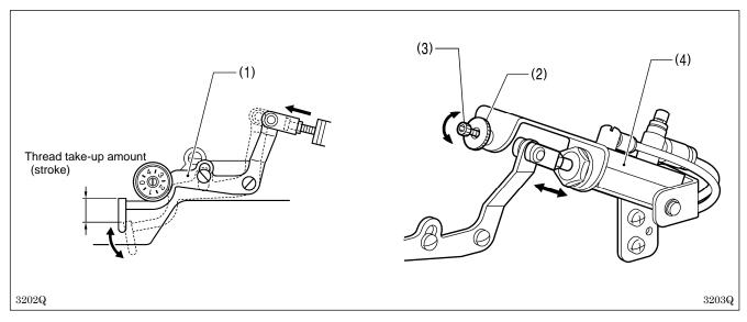
Loosen the nut (2) and move the stopper (bolt) (3) to adjust the protruding position of the cylinder (4).
