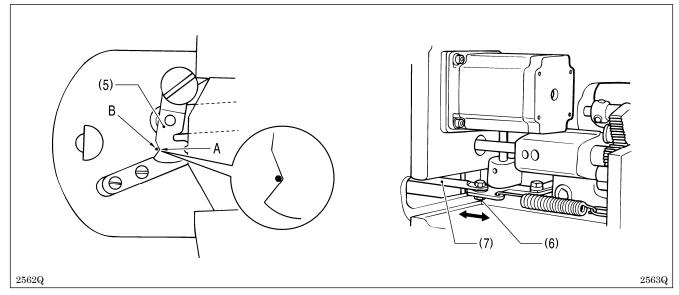
5. Loosen the nut (6) and move the connecting rod lever (7) to the left or right to adjust so that the V section A is aligned with the index mark B on the needle plate when in this condition (the procedure 3.) and the movable knife (5) is pushed to the machine pulley side so that there is no play.
