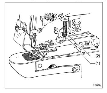
Loosen the adjusting nut (1) and turn the adjusting nut (2) to the point where it is just tight enough that the material will not slip out of place when it is slightly pulled (keep pressure as slight as possible).
