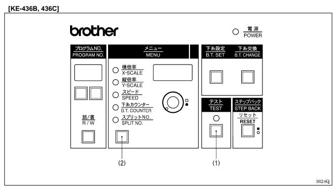
1. While pressing the TEST switch (1), turn on the power to the machine. Version number of each PROM can be confirmed.
