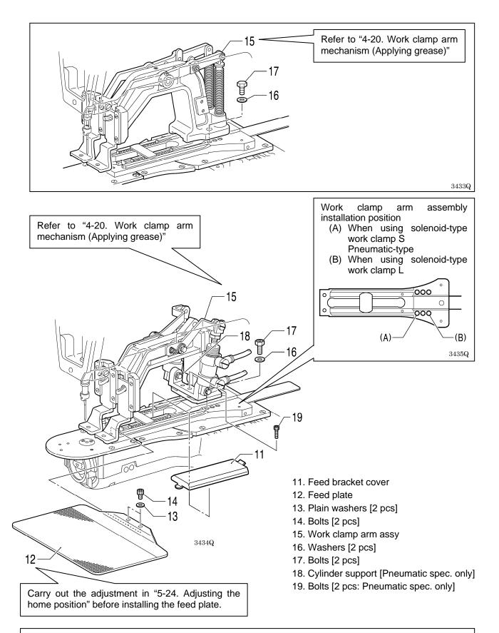
After installing, carry out test feeding and check that the needle hole is inside the work clamp and the feed plate frame. If the needle hole is not inside the frame, adjust the position of the work clamp arm assembly and feed plate.
