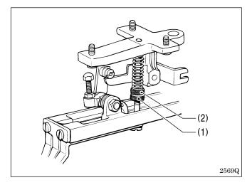
Loosen the lower adjusting ring (1) as much as possible (to the extent that the material being sewn does not slip and alter the pattern). Then, adjust the pressure by turning the upper adjusting ring (2).
