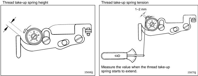
\* When the spring height (stroke) is great or the spring tension is insufficient, it may cause the thread end length to vary after thread trimming.
