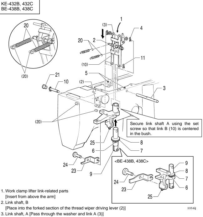
When assembling, apply grease to the required places while referring to "4-5-1. Applying grease".
