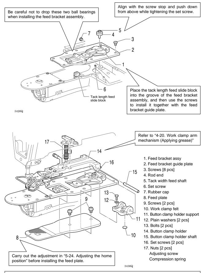
After installing, check that the needle passes into the button hole without touching the button. (Refer to "5-14. Adjusting the position of the button holder".)
