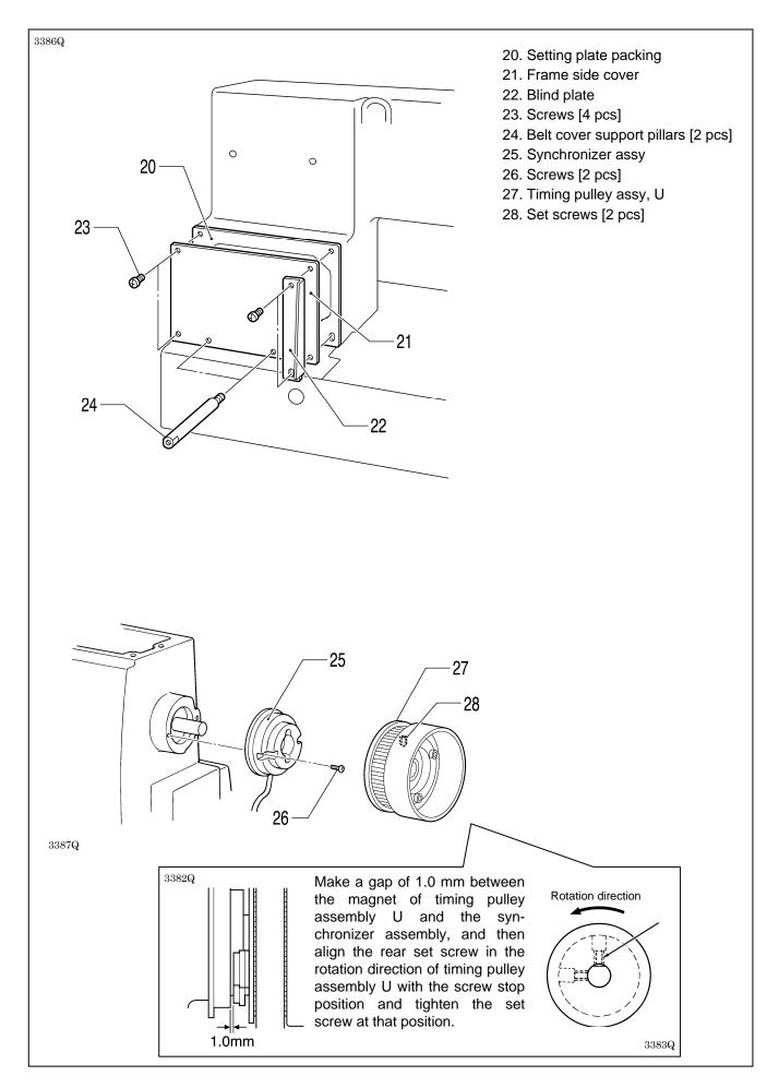
4 - 9. Stepping foot lifter mechanism (KE-435B, 435C, 436B, 436C)
