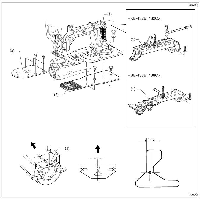
1. Remove the arm assembly (1), the feed plate (2) and the needle plate (3).
