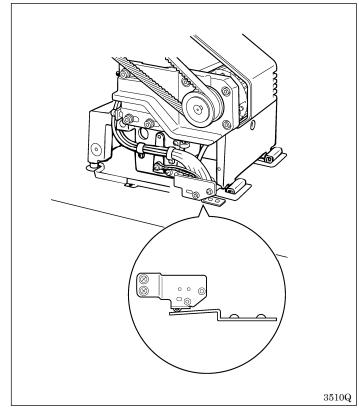
Check that the head position switch is turned on as shown in the illustration.
