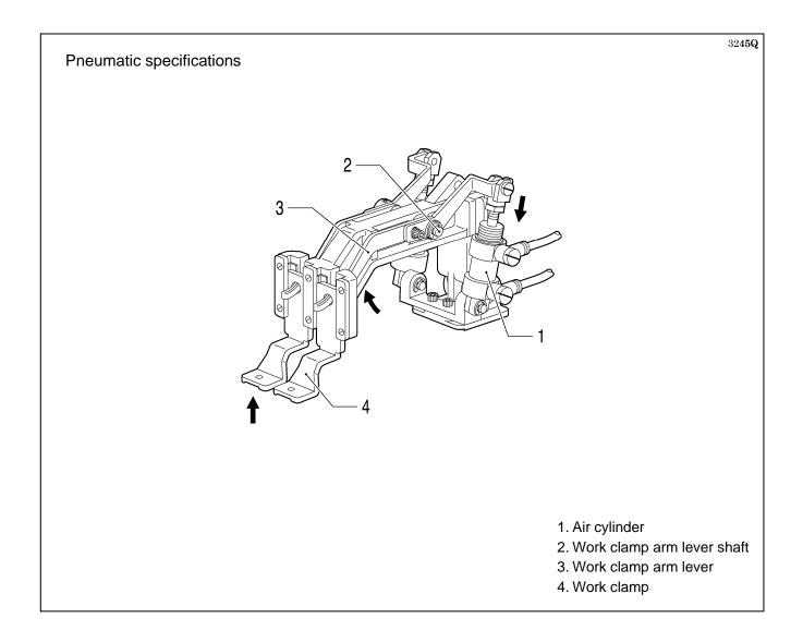
2-4. Work clamp open-close mechanism (KE-432B, 432C)
