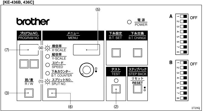
1. When the SPLIT NO. indicator (1) is illuminated and the R/W switch (3) is pressed while the TEST switch (2) is being pressed, the X-SCALE indicator (4) will illuminate and the state of the X home position signal will appear on the display screen (5).
