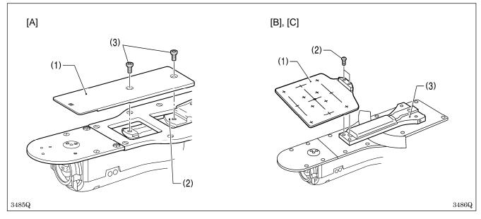
1. Install the home position standard plate (1) to the feed bracket (2) with the two screws (3).
