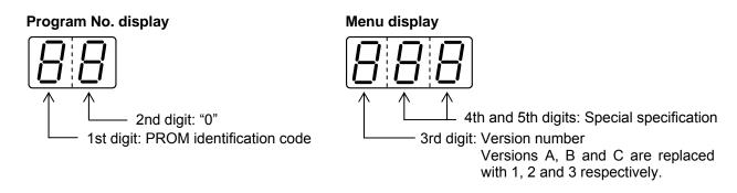
2. Every time the MENU switch (2) on the panel is pressed until the TEST switch (1) is pressed again, the indication will change as follows:
