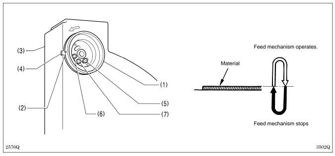
Loosen the screw (5) (at the U side on the pulley), and turn the pulley (1) so that the mark (2) on the pulley is inside the mark (4) of the belt cover (3). The pulley (1) will stop more slowly if the screw (5) is moved counter to the normal direction of rotation, and will stop more quickly if the screw (5) is moved in the normal direction of rotation.
