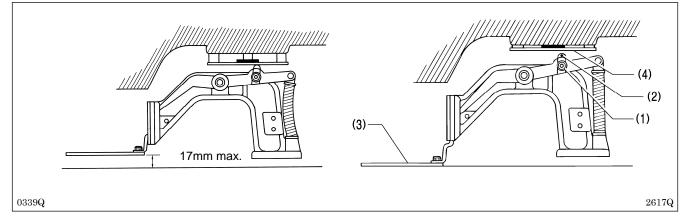
To adjust the work clamp lift amount, loosen the bolt (1) and move the presser arm lever plate (2) up or down.
