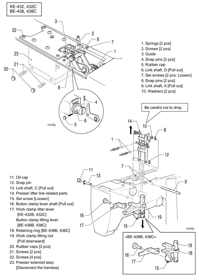
3 - 1 5. Stepping foot lifter mechanism (KE-435B, 435C, 436B, 436C)
