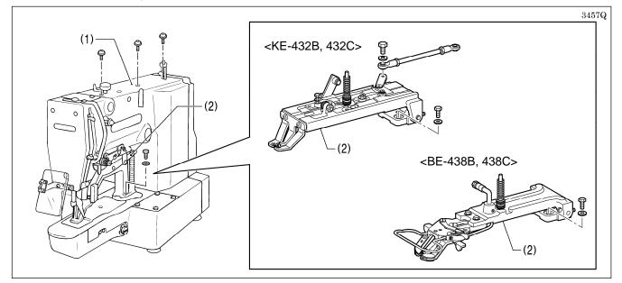
1. Remove the top cover (1) and the work clamp arm assembly (2). Remove the top cover (1) and the button clamp assembly (2). [BE-438B, 438C]
