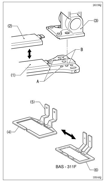
The work clamp for the BAS-311F can be used. Replace the feed bar guide cover (1) with the feed bar guide cover assembly, LL (2) (optional). Then, change the installation position for the presser arm assembly (3) from the standard installation position A to installation position B.
