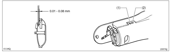
Turn the machine pulley to align the tip of the rotary hook with the needle center line. Then loosen the set screw (1) and turn the eccentric shaft (2) to adjust so that the clearance between the needle and the rotary hook is 0.01 - 0.08 mm.
