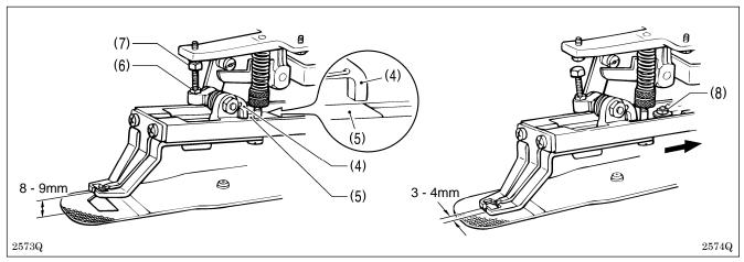
2. By loosening the nut (6) and turning the stop lever adjusting screw (7), adjust the stop lever (4) so that it separates from the stop position adjusting plate (5) when the work clamp is elevated 8 - 9 mm above the surface of the needle plate.
