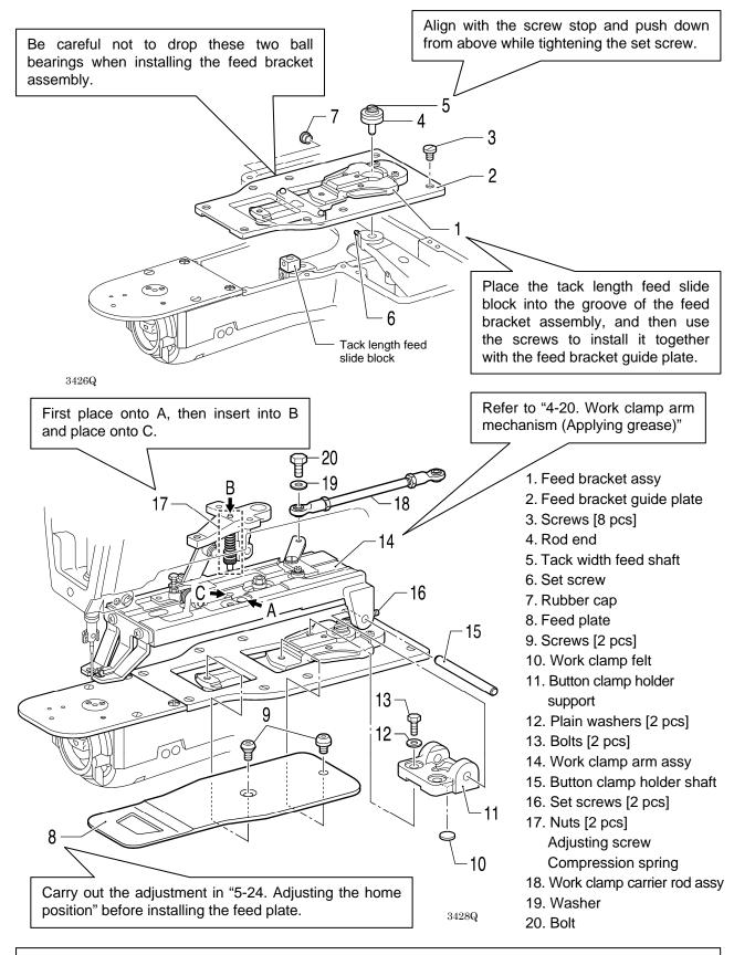
After installing, carry out test feeding and check that the needle hole is inside the work clamp and the feed plate frame. If the needle hole is not inside the frame, adjust the position of the button clamp holder support and feed plate.
