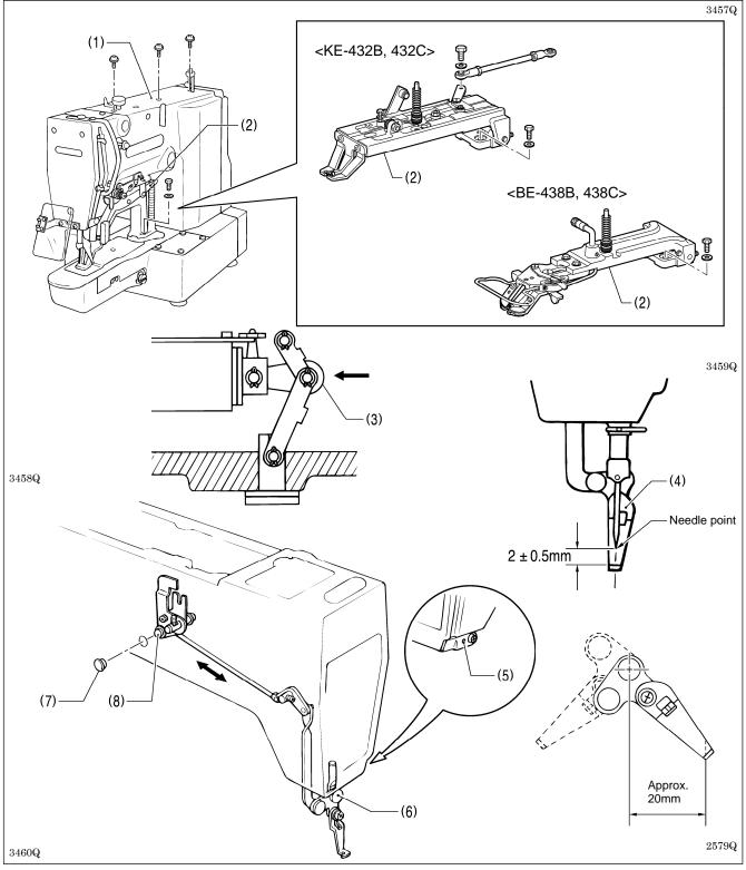
1. Remove the top cover (1) and the work clamp arm assembly (2).
