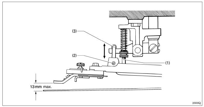
Remove the button clamp presser spring (1), loosen the screw (2) and adjust the button clamp holder hook (3) by moving it up and down.
