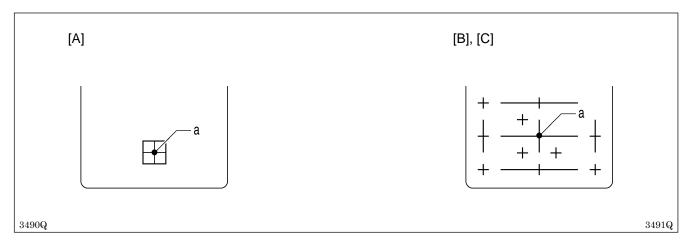
5. Turn the pulley by hand and check at what point the needle drops to the home position standard plate. If the needle does not drop to point (a), carry out the following adjustments. **Note:**
