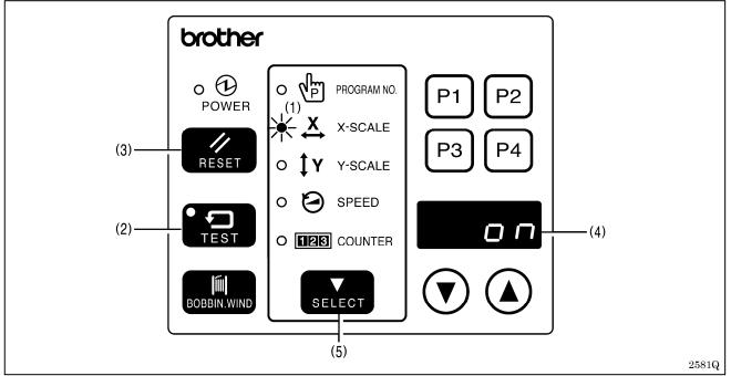
When the X-SCALE indicator (1) is illuminated and the RESET switch (3) is pressed while the TEST switch (2) is being pressed, the state of the X home position signal will appear on the display window (4).
