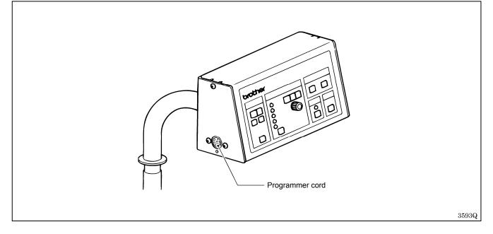
Programmer and programmer circuit board (KE-436B, 436C)
