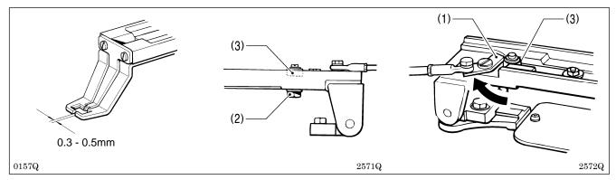
1. With the presser closing lever (1) pushed all the way by hand in the direction of the arrow in the illustration, loosen the nut (2) and move the presser closing roller (3) so that the gap is 0.3 - 0.5 mm when the work clamp is closed while the sewing machine is in operation.
