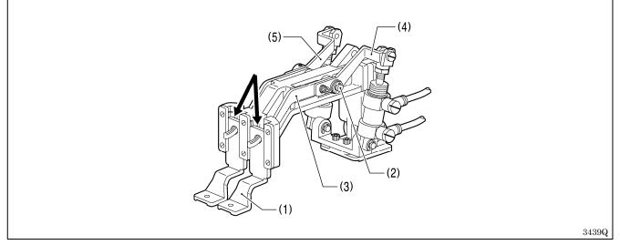
1. Sliding portion of the work clamp (1) (Apply small amount of grease.)
