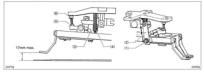
While the machine is stopped, loosen the bolt (1) and move the presser roller attachment plate (2) vertically to adjust the lift amount.
