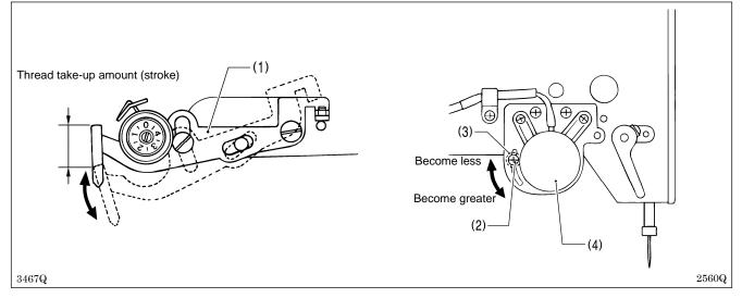
Loosen the screw (2) and move the stopper (3.57 nut) (3) to adjust the operating angle of the thread take-up solenoid (4).
