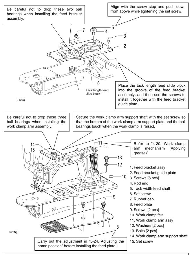
After installing, carry out test feeding and check that the needle hole is inside the work clamp and the feed plate frame. If the needle hole is not inside the frame, adjust the position of the work clamp arm assembly and feed plate.
