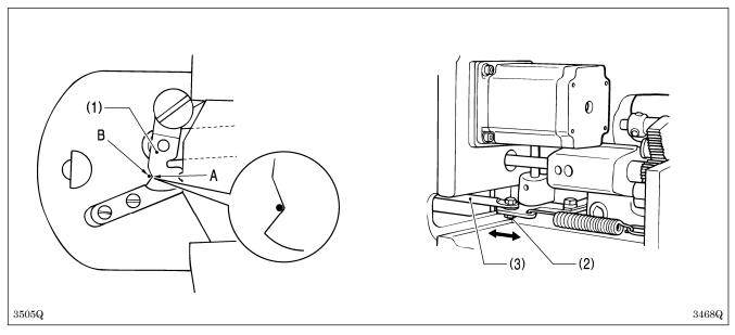
Loosen the nut (2) and move the connecting rod lever (3) to the left or right to adjust so that the V section A is aligned with the index mark B on the needle plate when the sewing machine in the stopped position and the movable knife (1) is pushed to the machine pulley side so that there is no play.
