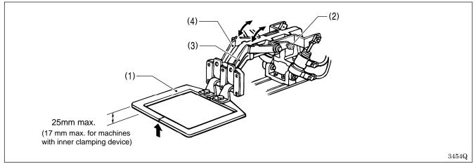
1. Raise the work clamp (1) and loosen the screws (2).
