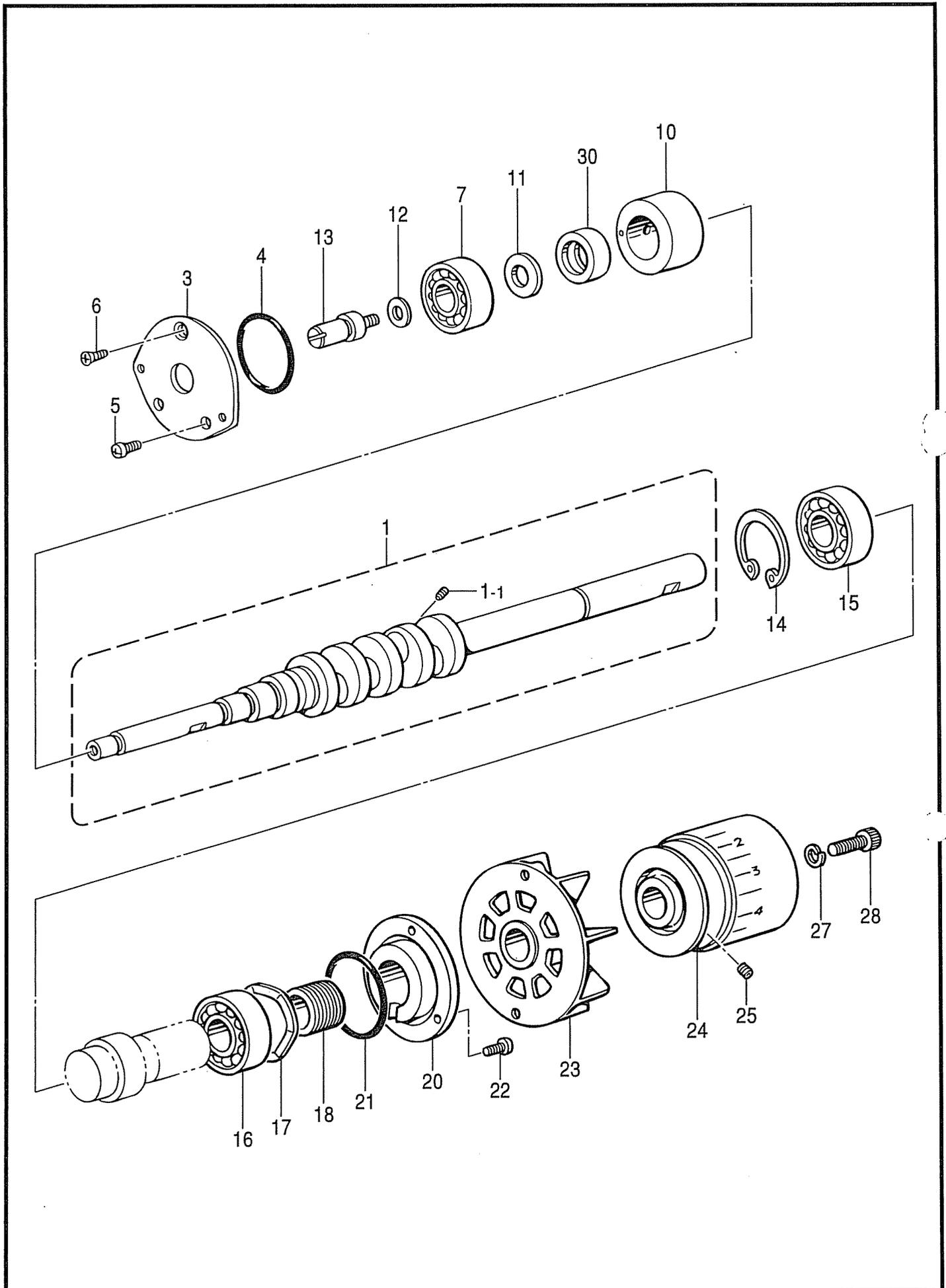
B. 駆動軸関係 / Crankshaft mechanism
