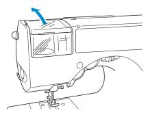
Push the thread cassette eject lever on the left side of the machine toward the back.
