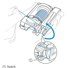
Pull the thread under the disc at the front in the lower-left corner and around to the right, and then cut the thread with the cutter.
