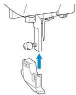
Hold the presser foot holder in place with your right hand, and then tighten the screw using the screwdriver in your left hand.
