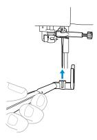
Lift up the needle-changing tool so that the fork hooks onto the needle clamp screw.
