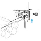
Using the screwdriver, loosen the needle clamp screw.
