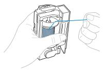
Pass the thread through the slit in the top of the thread cassette.
