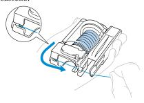
Pass the thread through the notch in the lower-right corner of the thread cassette, and then pull the thread to the left.
