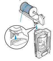
Thread the thread cassette with the thread from the spool on the extra spool pin.
