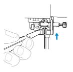
Insert the needle until it touches the needle stopper, and then use the screwdriver to tighten the needle clamp screw.
