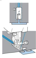
After sewing is finished, remove the paper.
