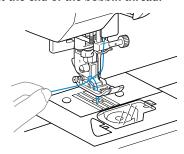
Pull out about 10-15 cm (3/8-5/8 inch) of the bobbin thread under the presser foot toward the rear of the machine.
