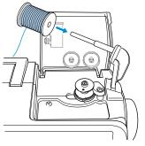
Slide the spool cap onto the bobbin thread spool pin.
