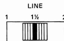
The amount of paper fed for each operation of the function keys (PAPER UP and PAPER DOWN) is 2.117 mm (1/12").
