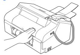
8 Push the paper tray firmly back into the machine. While holding the paper tray in place, pull out the paper support until it clicks and unfold the paper support flap. (See the illustrations in Loading paper and other media on page 13.)
