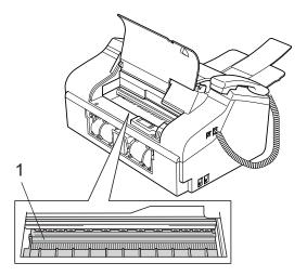
1 Clean the machine printer platen (1).
