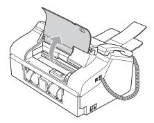
If you cannot remove the jammed paper from the front of the machine, or the error message still appears on the LCD after you have removed the jammed paper, please go to the next step. Remove the Lower Jam Clear Cover (1) from the back of the machine. Pull the jammed paper out of the machine.
