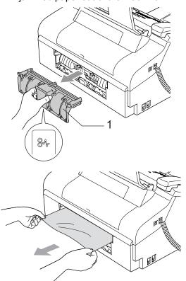
5 Put the Lower Jam Clear Cover back on. Make sure the cover is set properly.
