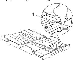
3 Press and slide the paper side guides (1) and paper length guide (2) to fit the paper size.
