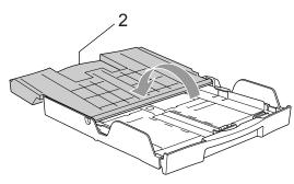
2 If you are using Letter, A4 or Legal size paper, press and hold the universal guide release button (1) as you slide out the front of the paper tray to match the paper size you are using.
