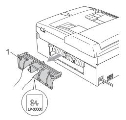
3 Clean the Paper Pick-up Roller (1) with isopropyl alcohol on a cotton swab.
