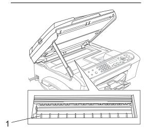
1 Clean the machine printer platen (1).
