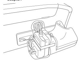
Route the AC power cord through the guide on the side of the machine. Then, plug the adapter into an AC power outlet.
