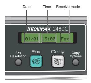
When the machine is idle (not being used) it will return to the default display shown above. The default display shows the date, time, and the current receive mode.
