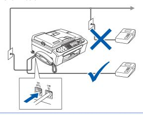
Set the receive mode to 'External TAD' for FAX-2480C, or 'Manual' for FAX-2580C if you have an external answering machine. For details, see Connecting an external TAD (telephone answering device) in Chapter 7 of the User's Guide.
