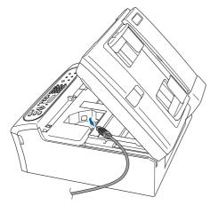
3 Carefully route the USB cable through the trench and out the back of the machine as shown below and connect the cable to your computer.
