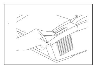
Press the control panel switch. The printer will start printing a test sample page.
