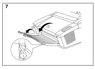
Open the output tray. (①) Extend the extension support wire. (②)
