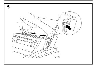
Pushing and sliding the tabs, move the paper guides to fit the paper width.
