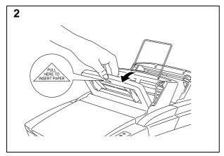
Open the cover of the multi-purpose sheet feeder 1.
