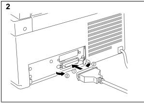
Connect the parallel interface cable (printer cable) to the parallel interface port of the printer. ( ① )
