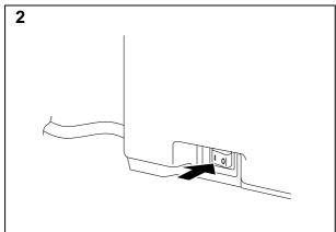
Turn on the power switch that is located on the left side of your printer.
