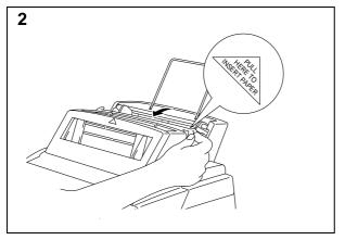
Open the cover of the multi-purpose sheet feeder 2.
