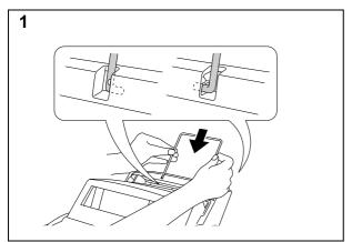
Install the paper support onto the rear multi-purpose sheet feeder 2.
