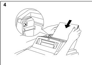
Load paper in the multi-purpose sheet feeder 2 with the printing surface face down.
