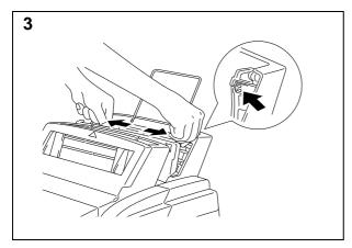
Pushing and sliding the tabs, move the paper guides horizontally to the widest position.
