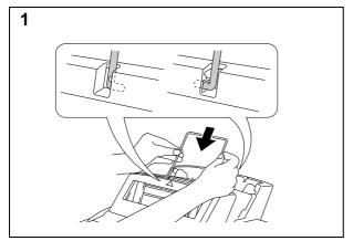
Install the paper support onto the front multi-purpose sheet feeder 1.
