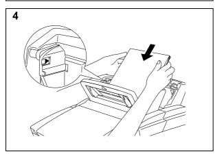
Load paper in the multi-purpose sheet feeder with the printing surface face down.
