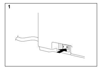
Make sure that the printer power switch is off before connecting or disconnecting the interface cable.
