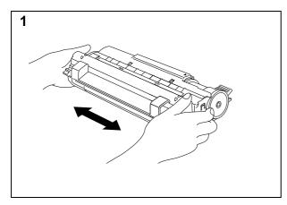
Unpack the drum unit assembly with the toner cartridge included. Gently shake it from side to side five or six times.
