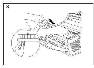
Holding the drum by its handles, install it into the printer. The drum will slide easily into place.
