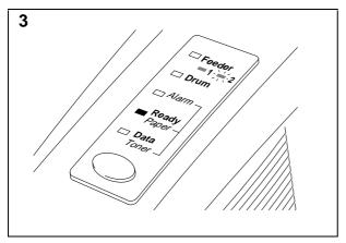
Make sure that the READY lamp is lit after the printer has warmed up (approximately 30 seconds).
