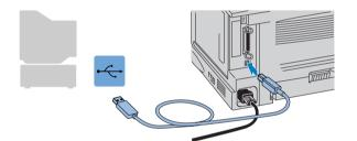
Connect the USB interface cable to your PC, and then connect it to the printer.
