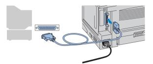
4 Connect the interface cable to your PC, and then connect it to the printer.
