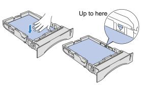
Load paper into the paper cassette. Check that the paper is flat in the tray and below the maximum paper mark.
