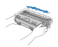
Unpack the drum unit assembly. Rock it from side to side 5 or 6 times to distribute the toner evenly inside the
