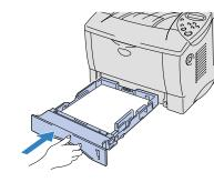
Re-install the paper cassette into the printer.
