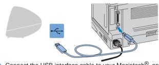
Connect the USB interface cable to your Macintosh<sup>®</sup>, and then connect it to the printer.
