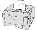
Press the Go switch. The printer prints a test page. Check that the test page is printed correctly.
