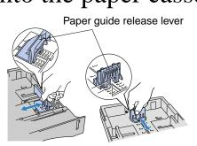
While pressing the paper guide release lever, slide the adjusters to fit the paper size. Check that they fit correctly into the slots.
