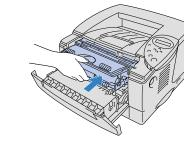
Install the drum unit assembly
