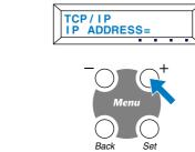
Press the + button until IP ADDRESS = is displayed. Press the Set button.
