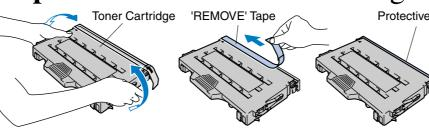
Pull off the tape labeled 'REMOVE,' and Rock the toner cartridge 3 then remove the orange protective cover.
