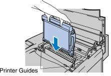
Insert the OPC belt cartridge into the printer guides with the flat side facing
