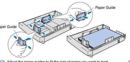
Adjust the paper guides to fit the size of paper you want to load. Load paper in the paper tray.
