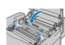
5 Lock the belt cartridge lock levers. Close the top cover.
