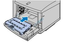
3 Install the toner cartridge by sliding it into the correct guide. Match the cartridge color label to the corresponding label
