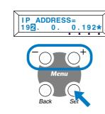
Enter the IP address of the printer using the + and - buttons. Press the Set button to go to next digit. Press the Set button to complete the IP address. An asterisk mark (\*) appears on the LCD.
