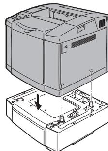
**4** Fit the two stopper fittings on the right and left hand sides of the Lower Tray Unit.
