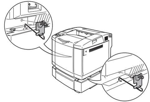
**5** Cover the gaps on the right hand side with the right-hand side cover by first inserting the hook at the back. Cover the gap on the left hand side with the left-hand side cover by first inserting the hook at the back. Close both of the side covers by putting the notch over the hook of the Lower Tray Unit.
