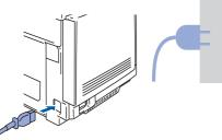
Plug the AC power cord into an AC power outlet/socket.
