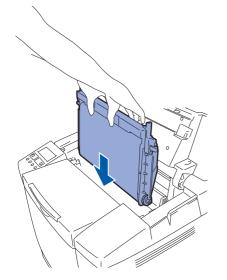
4 Lock the belt cartridge lock levers. Close the top cover.
