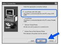
8 When this screen appears, make sure the printer's power switch is on. Connect the USB interface cable to your PC, and then connect it to the printer. Click the **Next** button.
