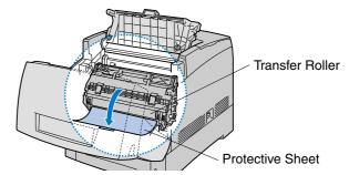
Remove the protective sheet Note: Do not touch the black surface of the transfer roller
