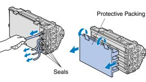
Pull the 4 seals firmly to remove them completely Remove the protective packing.
