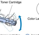
3 Insert the toner cartridge with the label side facing up. Match the cartridge color label to the corresponding label on the printer.
