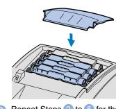
6 Repeat Steps 2 to 5 for the remaining toner cartridges. Put the top cover back on.
