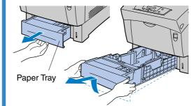
Pull the paper tray out until it stops. Lift up the front of the paper tray slightly and remove it from the printer
