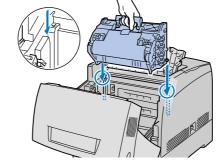
Align the rollers of the print head cartridge with the slots, and then gently lower it into the printer.
