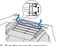
4 Turn the levers by pressing down firmly and lock them to the 🔒 mark.
