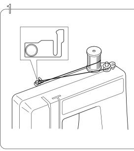
Place the thread spool on the spool pin and pass the thread around the bobbin winder thread guide.
