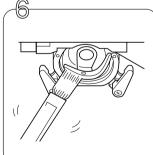
Remove any accumulated lint and thread with a brush.
