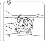
Holding the bobbin case by the latch align the finger with the top opening of the shuttle race , insert the case into the shuttle race and release the latch. The latch should hold the bobbin case in place.
