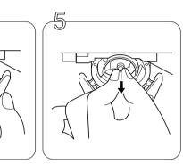
Remove the hook by grasping the center post and pulling out. Note it's position related to the driver.
