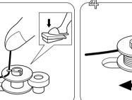
While holding the end of the thread, depress the foot controller.
