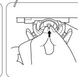
Grasp the center post of the hook, match the hook position opposite the driver and insert.
