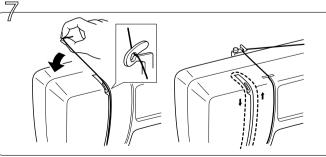
Guide the thread up the left channel, clear to the back of the opening around the take-up lever and back down the left side of the channel to thread the take-up lever.
