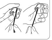
Pull the thread tail into the bobbin case groove, under the spring clip and into the thread guide hole.
