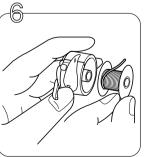
Hold the bobbin case as shown, insert the bobbin with the thread coming from the bottom toward the top and the thread tail hanging out of the bobbin case.
