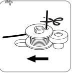
When the bobbin is full, it will stop winding. Cut the thread, slide the winding shaft to the left and remove the bobbin.
