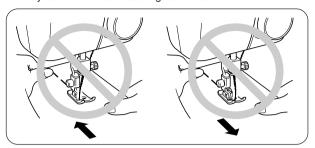
\*Do not turn the balance wheel and pull the fabric by force when the thread is entangled or the motor is locked. If the thread is entangled, remove the thread and fabric according to the procedure below.
