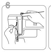
Grasp the thread on both sides of the tension disc and pull to ensure it is in place.
