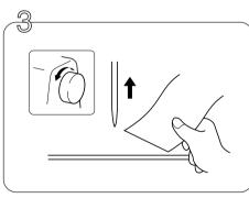
Turn the balance wheel to raise the needle. then remove the fabric.
