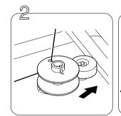
Pass the thread through the hole on the bobbin from inside, and slide the winding shaft to the right.
