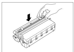
(4) Take the new refill roll of film from the sealed package. Remove the separator sheet. Holding the yellow colored plastic side holders of the film roll. Place the film into the cartridge as illustrated. The film can only be placed into the cartridge in the correct direction.
