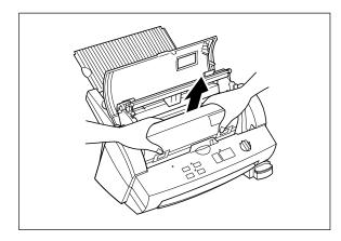
(1) Remove the film cartridge from the machine being careful not to grab the cartridge by the shutter.
