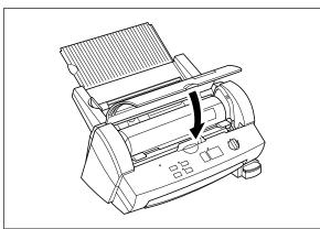
(10) Press the **Feed** button until you can see the edge of the film to remove any slack from the film.
