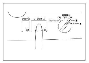
(4) Turn the POWER dial to Cutter Off, Border or No Border to select the cut mode.
