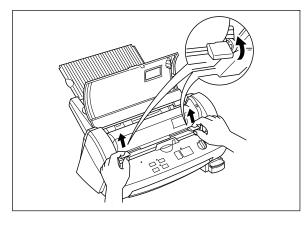
(4) Push the yellow colored tab of side cutter unit to release the lock as illustrated.
