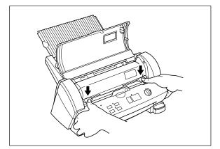
(10) Return the roller holder to its original position and press the roller holder levers as illustrated. You will hear the roller holder click into place.
