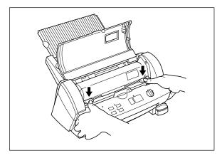
(4) Carefully install the new film cartridge, square end down, film slit facing towards the front of the machine.
