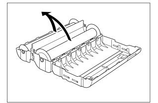
(3) Remove the old film roll from the cartridge.
