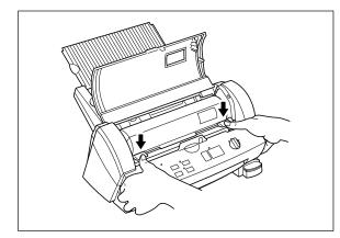
(5) Slide the old side cutter towards the center of the machine. Remove the side cutter.
