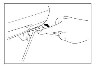
(1) Carefully insert a corner of the document all the way into the corner-cutter slot so that the corner of the laminated document is flush with the sides of the corner cutter.
