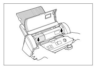
(4) Place the cartridge adapter into the machine as illustrated.
