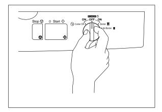
(3) Turn the power dial on the control panel to Cutter Off, Border or No Border. The green light on top of the **Start** button will light up. If the machine does not respond, check the connection of the AC adapter.
