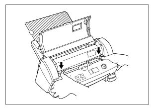
(8) Return the roller holder levers to its original position. Push until it clicks into place.
