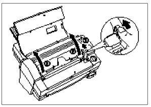
(3) Push the roller release lever (green color) and lift the roller holder upwards.
