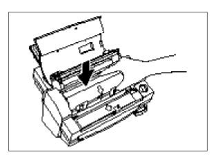
(3) Carefully install the film cartridge, square end down.
