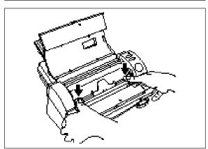
(10) Return the roller holder to the original position and press the roller holder lock buttons (purple color) as illustrated. You will hear the roller holder click into place. Press the roller holder further to secure the roller unit.
