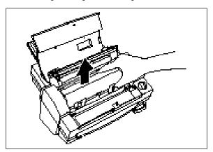
(1) Remove the film cartridge from the machine. Do not grab the shutter when removing the film cartridge from the machine.
