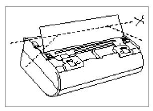
(6) Remove any excess laminating film by cutting along the engraved "cutting line" on the cartridge before reinserting the cartridge.
