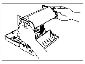
(4) Take the new roll of film from the sealed package. Holding the yellow colored plastic side holders of the film roll. Set the film into the cartridge as illustrated. The film can only be placed into the cartridge in the proper direction.
