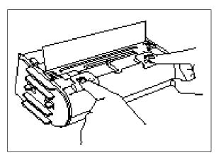
(6) Press on the two shutter catches marked "PUSH" to release the shutter.
