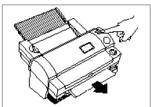
(2) Press "Feed" to feed the document manually. The "Feed" button is a self-repeating key. The document will continue to be fed until the "Feed" button is released. Keep pressing the "Feed" button until you see the end of the document.
