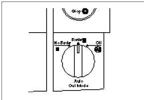
(4) Select the Cut Mode by using Auto Cut Mode selector switch.
