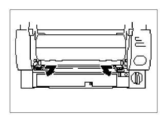
(5) Slide the old side cutter to the center. Remove the side cutter.
