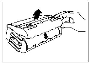
(5) Close the film cartridge. Make sure that the edge of the film sticks out of the film slit.
