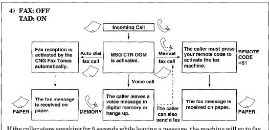
If the caller stops speaking for 5 seconds while leaving a message, the machine will go to fax receiving mode automatically.
