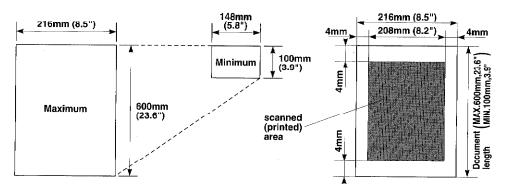
The size of the documents you want to send by fax should not be larger (or smaller) than your fax machine can accommodate. The documents should each be between 148 and 216 mm (5.8 and 8.5 inches) wide and between 100 and 600 mm (3.9 and 23.6 inches) long.
