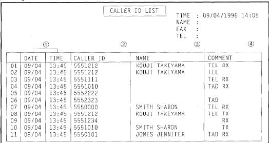
NOTE: "TX" means Transmit, "RX" means Receive.
