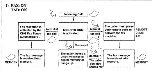
If the caller stops speaking for 5 seconds while leaving a message, the machine will go to fax receiving mode automatically.
