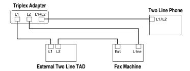
You can keep two-line telephones on other wall outlets as always. There are two ways to add a two-line telephone to the MFC's wall outlet. You can plug the telephone line cord from the two-line telephone into the L1+L2 jack of the triplex adapter. Or, you can plug the two-line telephone into the TEL jack of the two-line TAD.
