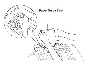
Press and slide the guide to fit the paper width.
