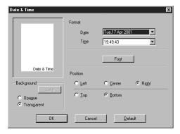
Click the Setting button to change the Date and Time Format, Position and Font. To include a background with the Date and Time, select Opaque. When Opaque is selected, you can click on the Color button to change the color of the Date and Time background.
