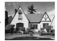
After the ink head nozzle is cleaned, the horizontal lines are gone.
