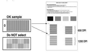
For 600 DPI, press the number of the test print that most closely matches the number 0 sample (1-8).
