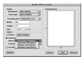
Perceptual Matching—All the colors of a given gamut are scaled proportionally to fit within another gamut. This intent pretty much maintain the balance between the colors in the image. This intent is the best choice for realistic images, such as scanned photographs.
