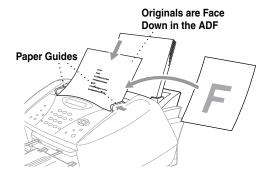
■ The automatic document feeder (ADF) can hold up to 20 pages, feeding each one individually through the MFC. Use standard (20 lb/75g/m²) paper when using the ADF.
