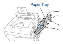
Attach the output paper support to the paper output slot, and then pull out the extension.
