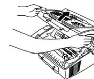
C. Holding the drum unit by its handles, insert it into the MFC.
