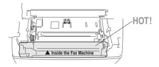
Open the top cover. Make sure the top cover is completely open. To remove the drum unit, hold each side of the drum by its handles and gently lift the drum forward toward you.
