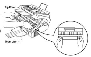
3 Remove the toner cartridge from the drum unit and keep it in a safe place. For more information, see Replacing the Toner Cartridge, page 15-26.
