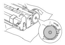
8 Reinstall the drum unit into the fax machine and close the top cover.
