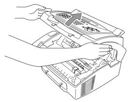
3 Holding the drum unit by its handles, insert it into the MFC.
