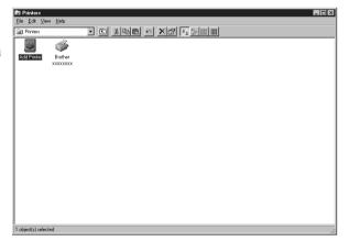
19 You will have to install the other drivers (such as scanner), manually. Click **Start** in the task bar, then select **Run**, and then type x:\nt40\setup\setup\setup.exe, and then click **OK**. ("x" is the drive letter for your CD-ROM drive.)
