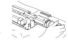
4 Unpack the new toner cartridge. Place the used toner cartridge into the aluminum bag and discard it according to local regulations.
