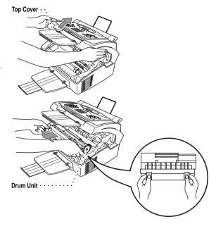
Place the drum unit on a drop cloth or large piece of disposable paper to
