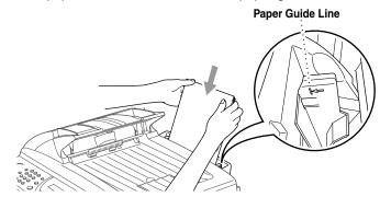
B. Press and slide guide to fit the paper width. Paper Width Guides
