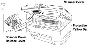
B. Pull the protective yellow bar out of the machine.
