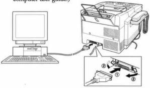
Before plugging the MFC in, plug your computer in and turn it on. Then, plug in the MFC.
