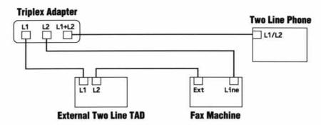
You can keep two-line telephones on other wall outlets as always. There are two ways to add a two-line telephone to the MFC's wall outlet. You can plug the telephone line cord from the two-line telephone into the L1+L2 jack of the triplex adapter. Or, you can plug the two-line telephone into the **TEL** jack of the two-line TAD.
