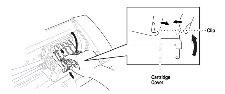
6 Remove the ink cartridge by lifting it up and out of the print head.
