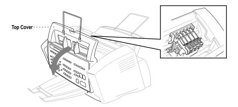
**3** Open the ink cartridge covers by pressing the clips together as shown in the illustration.
