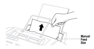
Pull the jammed paper upward and remove it.
