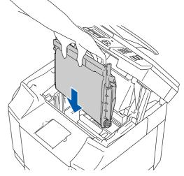
5 Lock the belt cartridge lock levers.
