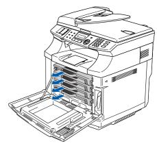
Carefully pull the protective part out of the machine.
