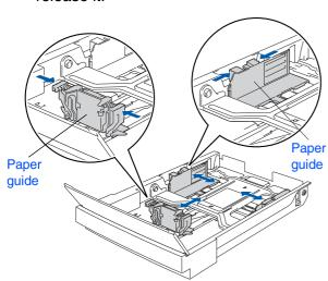
4 Fan the stack of paper well to avoid paper jams and misfeeds.
