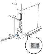
2 Plug the AC power cord into an AC outlet. Turn the power switch on.
