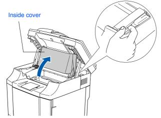
3 Remove the orange belt tension release pins from both sides of the OPC belt cartridge. Remove the protective sheet.
