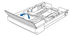
3 Squeeze the snap lock on the end of the front paper guide. Slide the front paper guide to the position for the size of paper you are using. Release the snap lock. Squeeze and slide the left hand side paper guide to the paper size you are using, and release it.
