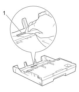
3 Lift the green Jam Clear Flap (1), and then clean the Paper Pick-up Rollers (2) with a soft lint-free cloth moistened with water.
