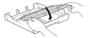
2 Gently put the paper into the paper tray printing surface face down.Check that the paper is flat in the tray.
