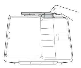
2 Slide the manual feed slot paper guides to match the width of the paper you are going to use.
