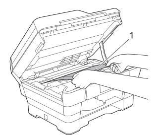
8 Move the print head (if necessary) to take out any paper remaining in this area. Make sure that jammed paper is not left in the corners of the machine (1) and (2).
