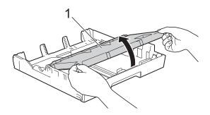
5 Gently press and slide the paper length guide (1) to fit the paper size. Make sure that the triangular mark (2) on the paper length guide (1) lines up with the mark for the paper size you are using.
