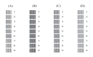
5 For the "A" pattern, swipe up or down, or press ▲ or ▼ to display the number of the test print that has the least visible vertical stripes (1-9), and then press it. Press OK.
