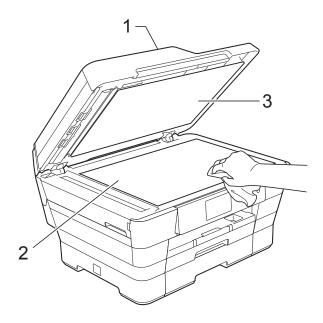
3 In the ADF unit, clean the white bar (1) and the glass strip (2) with a lint-free cloth moistened with a non-flammable glass cleaner.
