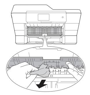
5 Make sure you look carefully inside the machine above and below the green Jam Clear Flap for any pieces of paper.
