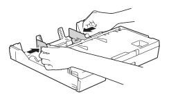
3 Put envelopes in tray #1 with the printing surface face down. If the envelope flaps are on the long edge, load the envelopes with the flap on the left, as shown in the illustration. Gently adjust the paper side guides (1) to fit the size of the envelopes.
