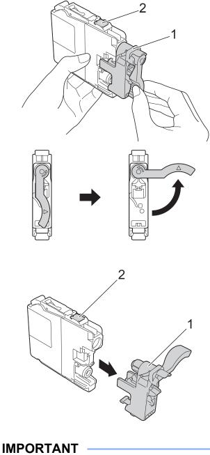
DO NOT touch the cartridge in the area indicated (2); this can prevent the machine from detecting the cartridge. 5 Each color has its own correct position. Insert the ink cartridge in the direction of the arrow on the label.
