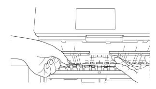
6 Using both hands, use the finger holds on each side of the machine to lift the scanner cover (1) into the open position.
