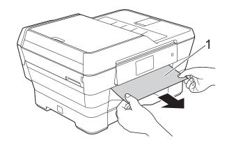
Lift the green Jam Clear Flap, and remove the jammed paper.
