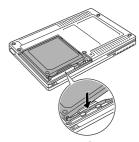
4 Install the battery cover by sliding it onto the back of the MW-145BT.
