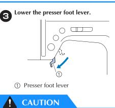
• Before replacing the needle, place fabric or paper under the presser foot to prevent the needle from falling into the hole in the needle plate.
