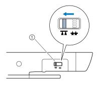
Feed dog position switch (as seen from the rear of the machine)
