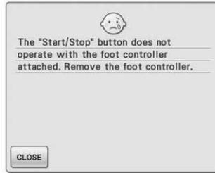
This message is displayed when the "Start/Stop" button is pushed to sew Utility stitches or Character/Decorative stitches while the foot controller is connected. (This message does not appear when embroidering).
