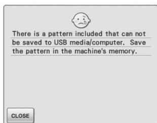
This message is displayed when you try to save a copyright protected pattern to USB media/Computer. According to copyright laws, patterns that are illegal to reproduce or edit cannot be saved to USB media or computer. If this message displays, save the pattern in the machine's memory.
