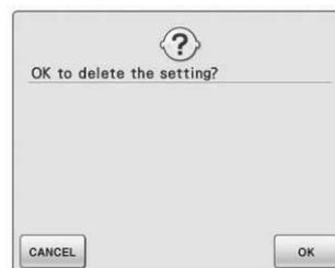
This message appears when **DELETE** or **ALL DELETE** is pressed to delete the settings for a utility stitch. To delete the selected settings, press **OK**.
