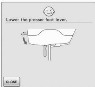
This message is displayed when the "Presser Foot Lifter" button is pushed while the presser foot lever is raised/ the needle is lowered.
