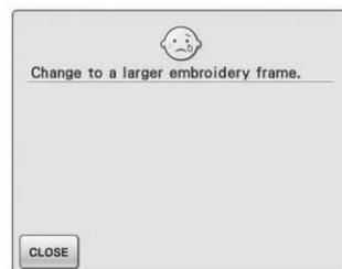
This message is displayed when the machine is in embroidery mode and the small frame is attached, and the selected pattern does not fit in the small frame. This message appears when embroidery frame (small) is attached while aligning the embroidery position using the built-in camera.
