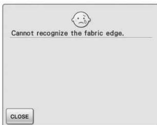
This message is displayed when the "Start/Stop" button is pressed before the edge of the fabric is detected. To detect the edge of the fabric using the built-in camera, press **CLOSE**, raise the presser foot, and then perform the operation again. (see page 148)
