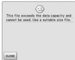
This message is displayed when the file size exceeds the data capacity of the machine. Confirm the file size and format. (see page 40.)
