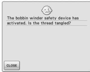
This message is displayed when the bobbin is being wound, and the motor locks because the thread is tangled, etc.
