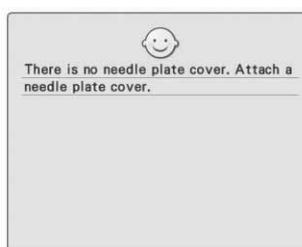
This message is displayed when the needle plate cover is not attached.
