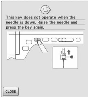
This message is displayed when a key on the LCD display is touched while the needle is in the down position.
