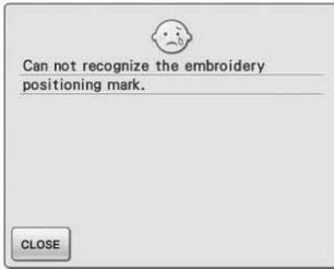
This message is displayed when the machine failed to recognize the embroidery positioning mark.
