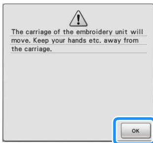
→ The built-in camera automatically searches for the embroidery positioning sticker, and then the carriage is moved so that the center of the embroidery pattern is aligned with the center of the embroidery positioning sticker. Regardless of the setting selected in the machine settings screen, the brightness of the light changes to “5” while the built-in camera searches for the embroidery positioning sticker.
