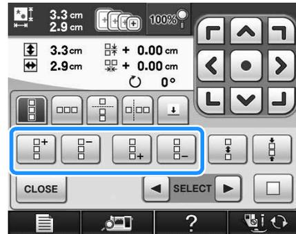
**5** Adjust the spacing of the repeated pattern.
