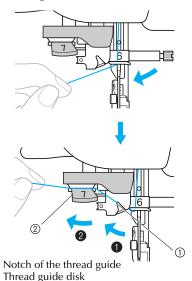
Cut the thread with the cutter on the left side of the machine.
