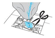
Remove the bobbin case. If threads remain in the bobbin case, remove
