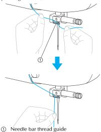
Next, use the needle threader to thread the needle. Continue with the procedure in "Threading the upper thread" (page 34).
