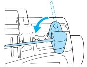
Place the upper thread spool for the needle on the right side onto the extra spool pin, and then secure it with the spool cap. The thread should unroll from the top front of
