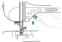
■ If thick seams are being sewn and the fabric does not feed at the beginning of stitching Zigzag foot "J" is equipped with a feature that keeps the presser foot level.
