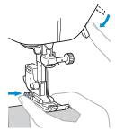
Release the button. The foot will lock in place level with the seam, allowing the fabric to feed.
