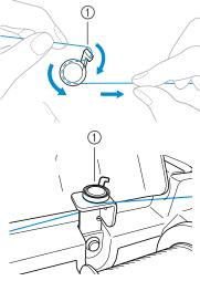
1) Thread guide for bobbin winding
