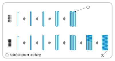
Determine the desired length of the darning. Set the button guide plate on buttonhole foot "A" to the desired length. (The distance between the markings on the presser foot scale is 5 mm (3/16 inch).)
