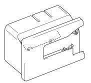
• The knee lifter can be stored attached to the bottom of the wide table.
