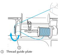
Pass the thread under the hook on the thread guide, and then wind it counterclockwise under the pretension disk.
