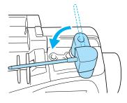
Place the upper thread spool for the needle on 6 the right side onto the extra spool pin, and then secure it with the spool cap.
