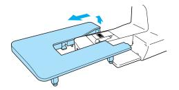
Install the flat bed attachment back in its original position.
