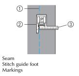
Aligning the fabric with a needle plate marking The markings on the needle plate show the distance from the needle position of a seam sewn with the straight stitch (left needle position). Sew while keeping the edge of the fabric aligned with a marking in the needle plate. The distance between the markings in the upper scale is 1/8 inch (3 mm) and the distance between the markings in the grid is 5 mm (3/16 inch).
