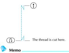
Reverse/reinforcement stitches WILL NOT be sewn and the thread will not automatically be cut until () ("Reverse/ Reinforcement Stitch" button) is pressed.
