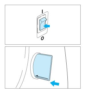
1. Set the main power switch to "**O**" to turn off the sewing machine.
