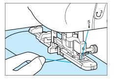
6. Gently hold the end of the upper thread, and then press the start/stop button to start the machine. Once sewing is completed, the machine automatically sews reinforcement stitches, and then stops.
