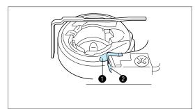
1. Set the main power switch to "**O**", and then remove the presser foot holder and the needle.
