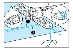
Π When sewing on stretch fabric with stitches over a gimp thread.
