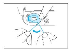
3. Guide the thread through the groove, then pull the thread toward you to cut off any excess.
