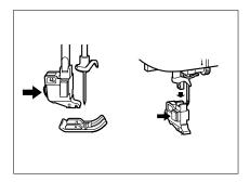
1. Remove the installed presser foot and the presser foot holder.
