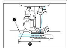
1. Set the stitch length to 5/32" (4.0 mm) and select a weak thread tension.
