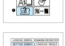
This sewing machine is equipped with a convenient guide that displays information and instructions on various operations, such as bobbin winding, upper threading, and LCD adjustment, making this machine easy to use.
