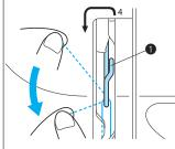
5. Pass the thread through the wire loop, and then lower the
