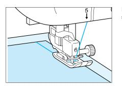
Place thin paper or stabilizer material under the fabric before sewing.
