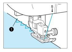
Sew the overcasting along the edge of the fabric with the needle dropping off the edge of the fabric at the right. • Needle drop point
