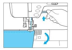
When you reach the corner, leave the needle in the fabric, raise the presser foot lever, and then turn the fabric. Lower the presser foot lever and continue sewing.
