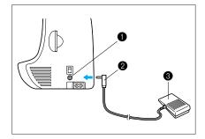
This foot controller (model N5V) is designed for use with this sewing machine (model PC-6500).
