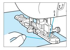
Gently hold the end of the upper thread, and then start sewing. Feed the fabric carefully by hand while the buttonhole is sewn. Once sewing is completed, the machine automatically sews reinforcement stitches, and then stops.
