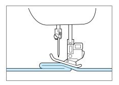
If the presser foot angles up as it approaches a thick seam, leave the needle in the fabric and raise the presser foot lever. After levelling off the sewing area by placing a piece of folded fabric or cardboard under the back of the presser foot, lower the presser foot lever and continue sewing.
