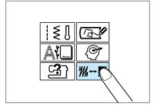
1. Press the **STITCH ADJUST** key, and then select the eyelet size.
