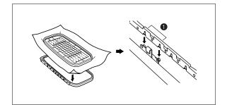
3. Stretch the fabric between the inner and outer embroidery frames while making sure that the reference lines on the embroidery sheet remain aligned with reference lines for the design drawn on the fabric. Then, attach the embroidery frame to the embroidery arm at the top installation position. (Refer to pages 90 - 92 for more details on attaching the embroidery frame.)
