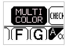
Before starting to embroider, press the MULTI COLOR key so that it appears as to turn on multi-color embroidering. After a character is embroidered, the machine automatically sews reinforcement stitches, and then stops so that the thread can be changed.
