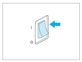
To turn on the machine, set the main power switch to "I". To turn off the machine, set the main power
