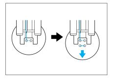
First, sew the two holes which are closest to you. Once they have been sewn, raise the presser foot lever, move the fabric so that the needle goes into the next two holes, and then sew them in the same way.
