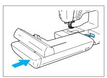
3. Insert the connector on the embroidery unit firmly into the connecting slot.
