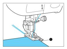
Attach presser foot  ${\bf G},$  lower the presser foot lever, and then sew the overcasting with the fabric edge against the guide of presser foot  ${\bf G}.$
