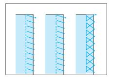
Attach presser foot J, and check that the needle drops slightly off the edge of the fabric before sewing.
