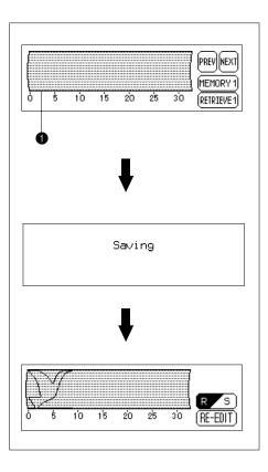
3. When an empty memory appears on screen, press that **MEMORY** # key to save your design. If a pattern has already been saved in memory address 1, it is displayed on the screen. Pressing the **MEMORY** key of a full memory will cause its contents to be placed by what you are saving.
