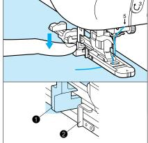
5. Gently hold the end of the upper thread, and then press the start/stop button to start the machine. Once sewing is completed, the machine automatically sews reinforcement stitches, and then stops.
