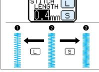
Press the STITCH ADJUST key, and then use the STITCH **LENGTH** keys [L] and [S] to adjust the stitch length of the bar tack.
