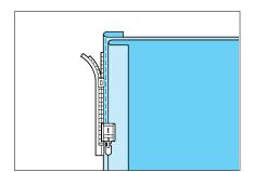
4. Attach the presser foot holder to the left pin of presser foot I, open the zipper, and then sew the bottom layer to the zipper from the top to base of the zipper.
