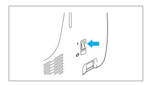
3. Set the main power switch to "I" to turn on the sewing machine.
