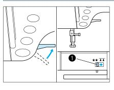
Raise the presser foot lever and slide the feed dog position switch to the right to lower the feed dogs.
