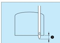
4. Check that the needle drops at the corner of the pocket, and then move the pocket back 5/64" (2.0 mm). 1 5/64" (2.0 mm)
