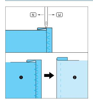
Press the STITCH ADJUST key, and then use the STITCH WIDTH keys wand N to adjust the needle position so that the needle slightly catches the fold of the hem.
