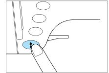
3. Press the **BACK** key to move back a few stitches slightly before the point where the thread broke.
