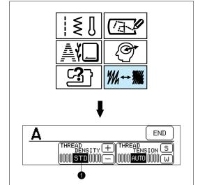
The thread density of characters and some frame patterns can be adjusted so that they are either coarser or finer when they are embroidered.
