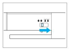
With the accessory compartment removed, the feed dog position switch can be seen at the base of the machine. To lower the feed dogs, for example when sewing buttons, slide the lever to the right. To continue sewing while the feed dogs feed the fabric, slide the lever to the left.
