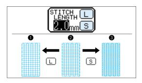
Press the **STITCH ADJUST** key, and then use the **STITCH LENGTH** keys L and S to adjust the stitch length of the darning.
