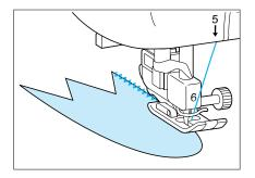
Before sewing an appliqué, attach it to the fabric either with adhesive or by basting it. Sew the zigzag stitch so that the needle drops off the edge of the appliqué.
