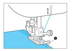
Baste the fabric beforehand and sew along the basting using a stretch stitch ( or Basting
