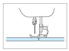
2. If the fabric does not feed at the beginning of sewing, place a piece of folded fabric or cardboard under the back of the presser foot to raise it.
