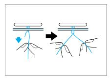
4. Gently hold the end of the upper thread, turn the balance wheel to check that the needle correctly goes into each hole in the button, and then start sewing. Once sewing is completed, the machine automatically stops.
