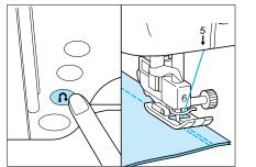
7. When the end of the stitching is reached, press the reverse/reinforcement stitch button to sew reverse stitches and stop the machine.
