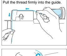
4. While holding the spool thread with your right hand, use your left hand to keep the thread taut while passing it through the guides as shown.
