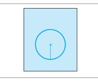
Create a frame pattern, and then embroider it. A cross (+) is sewn in the center of the frame after it is embroidered. This mark can be used as a guide for positioning characters or other patterns within the frame.
