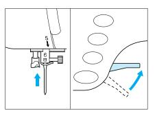
1. If the upper thread has broken: Stop the sewing machine, raise the needle and the presser foot lever, and then re-thread the upper thread.
