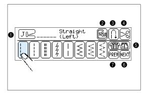
Press a key on the screen with your finger to select the pattern displayed inside the key or to start the indicated function or operation.
