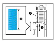
1. Attach buttonhole foot **A** and set the scale to the desired length of the darning.
