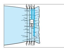
4. Attach presser foot **J**, press , and sew over the straight stitches.
