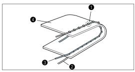
The upper thread and the bobbin thread should cross at about the center of the fabric. If the thread tension is incorrectly set, flat attractive stitches will not be sewn or the fabric will pucker. The thread tension for each stitch is preset to the most appropriate setting. However, in the following cases, the thread tension may need adjustment:
