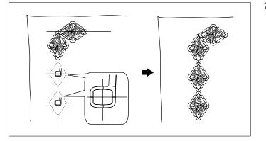
7. Before embroidering the bottom two patterns shown in the illustration, press the LAYOUT key, and position the pattern correctly. To position the frame so that the pattern will be embroidered correctly, press so that it appears as so that it appears as so the arrow keys to align the needle with the center of each pattern's reference lines (refer to page 105).
