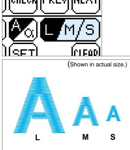
The size of the characters can be changed by pressing  $\Box$  M/S. Each time this key is pressed, it selects a different character size. Changing the character size changes the size of all characters in the text. When this key appears as  $\Box$  M/S, all characters are changed to the large size. When the key appears as  $\Box$  M/S, all characters are changed to the medium size. When the key appears as  $\Box$  M/S, all
