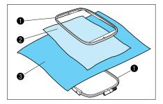
Using stabilizer material is an important part of creating attractive embroidery. It is particularly important when embroidering stretch fabrics, thin fabrics, and fabrics with coarse weaves. If necessary, two layers of stabilizer material may be attached.
