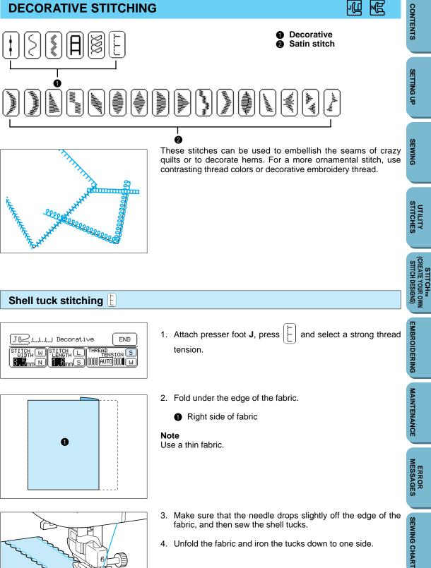
4. Unfold the fabric and iron the tucks down to one side.
