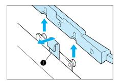
While pushing the release lever on the frame holder to the left, lift the embroidery frame up to remove it.
