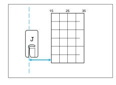
Align the edge of the material with a line on the needle plate to sew even seam allowances.
