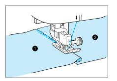
Fold over the desired width of the top fabric and position it over the lower fabric. Then, sew the zigzag stitch so that the stitching bridges both pieces of fabric.
