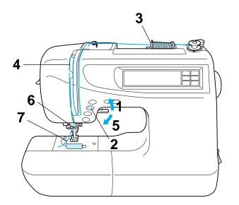
Raise the presser foot lever. (If the presser foot is not raised, the sewing machine cannot be threaded correctly.)
