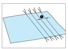
Press [] [Straight (Left)], set the stitch length to 5/32"(4.0 mm), and select a weak thread tension.
