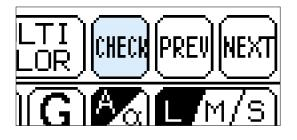
After a lot of text has been typed in, it may not be possible to view some of it on the screen. Press the **CHECK** key for the entire text to scroll across the screen.
