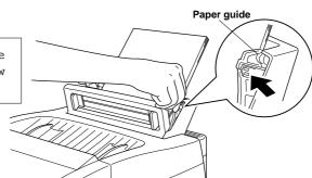
6) Attach the dust cover to the multipurpose sheet feeder cover.
