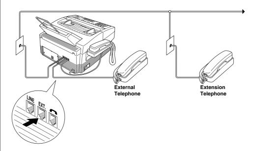
If the external telephone is in use, the warning message EXT. TEL IN USE will be displayed on the fax LCD. When the handset on the fax machine is picked up, an alarm will sound. You can disconnect the external phone and switch to the fax machine's handset by pressing  $\bf{Hook}$ .
