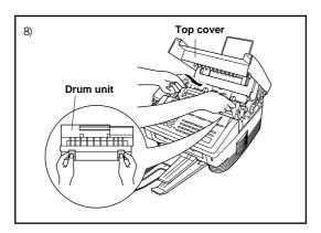
8) Holding the newdrum unit by its handles, install it. Close the top cover.
