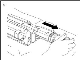
4) Remove the old toner cartridge from the drum unit by gently pulling it out.
