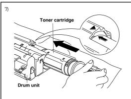
7) Slide the new toner cartridge into the opening on the right hand side of the drum unit. To ensure that the toner cartridge and drum unit fit together correctly, make sure the toner cartridge guide bar is exactly aligned with the guide slot in the drumunit.
