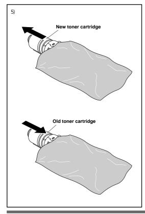
5) Unpack the new toner cartridge. Place the used toner cartridge into the aluminum bag and discard it according to local regulations.
