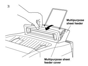
4) Load paper into the Multipurpose sheet feeder.
