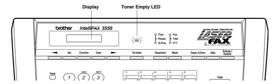
The Toner Empty LED will light and the display will show CHANGE TONER and TONER EMPTY alternately to indicate that the toner is empty. Once this indication appears, your machine will not resume printing until you have installed a new toner cartridge.
