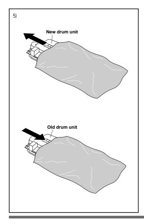
5) Wait to unpack the new drum unit until immediately before installing it. Place the old drum unit into the aluminum bag and discard it according to local regulations.
