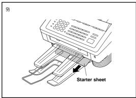
9) Turn on the power switch or plug in the power cord. The machine automatically will eject the starter sheet.
