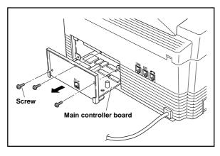
2. Unscrew the three screws securing the main controller board plate and pull out the board.
