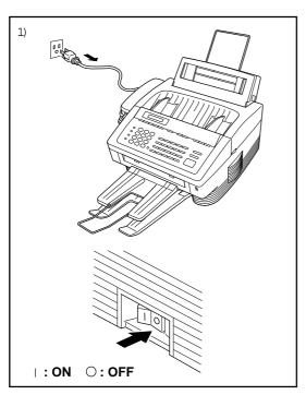
1) Turn off the power switch and unplug the power cord.
