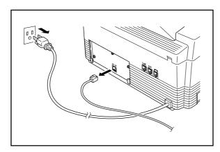
1. Unplug the power cord from the AC outlet and disconnect the interface cable.
