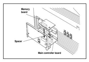
To install the memory board onto the main controller board, use the attached spacer and plugit into the lower right connectors of the main controller boards.
