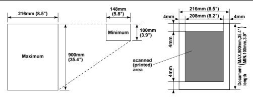
The size of the documents you want to send by fax should not be larger (or smaller) than your fax machine can accommodate. The documents should each be between 5.8 and 8.5 inches (148 and 216 mm) wide and between 3.9 and 35.4 inches (100 and 900 mm) long.
