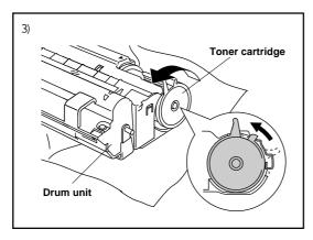
3) Gently turn the lever on the toner cartridge forward until it stops. The toner cartridge can not be removed unless the shutter is completely closed, by turning the lever fully to the front.
