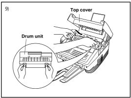
9) Reinstall the drumunit into the machine and close the top cover. Then, turn on the power switch or plug in the power cord.
