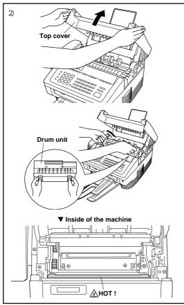
2) Open the top cover. To remove the drum unit, hold each side of the drum by its handles and gently lift the drum forward toward you.
