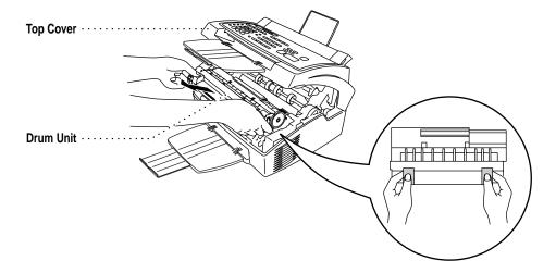
Remove the toner cartridge from the drum unit and keep it in a safe place. For more information, see "Replacing the Toner Cartridge" on pages 112–116.
