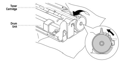
**3** Remove the old toner cartridge from the drum unit by gently pulling it out.
