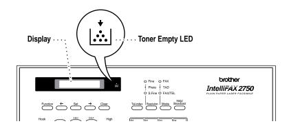
The Toner Empty LED light stays on and the display shows TONER EMPTY to indicate that the toner is empty. Once this indication appears, your fax machine will not resume printing until you have installed a new toner cartridge.
