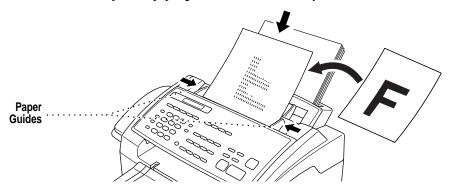
■ The FAX 2750's automatic document feeder (ADF) can hold up to 20 pages, feeding each one individually through the fax machine. Use standard (14 lb–24 lb) paper when using the ADF; if you're using heavier paper, feed each sheet individually to prevent paper jams.
