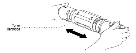
6 Slide the new toner cartridge into the opening on the right side of the drum unit. To ensure that the toner cartridge and the drum unit fit together correctly, make sure that the toner cartridge guide arrow is exactly aligned with the guide arrow on the drum unit.
