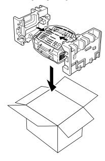
Place documents (manual and printed material) and the drum unit and toner cartridge assembly into the original carton as shown below:
