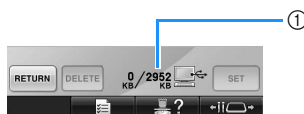
① Shows the amount of free space in the USB area of the machine. If pattern data with this size is added, it can be recalled (temporarily written).
