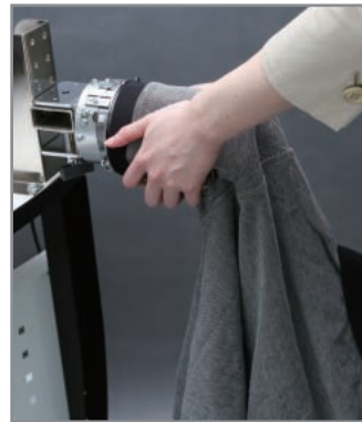
Stretch the piece over the special frame
