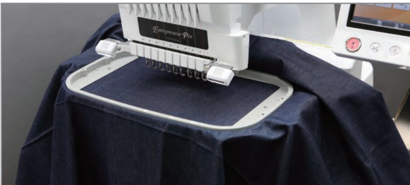
Cloth outside of the frame is kept on top of the frame and out of the way
