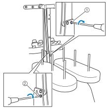
Insert screw and tighten.
