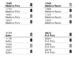
■ Expanded thread color display feature enables colors to be displayed as realistic true color The colors and thread color numbers are stored in the machine's memory. From this thread color library, you can select colors to create your own color thread table. If the pattern colors are changed using this table, the pattern can be displayed with only the thread colors that you have. In addition, the embroidery pattern can be displayed as it would appear after it is embroidered.
