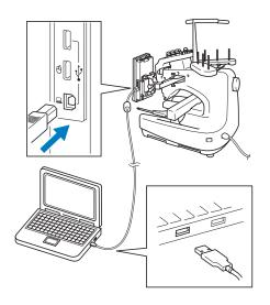
If the machine is positioned at a distance that the USB cable does not reach the computer, embroidery patterns can be transferred from the computer by temporarily saving them on USB media, which is then connected to the machine. Refer to "USB media" on page 160.
