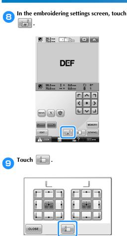
The needle bar is positioned in the lowerleft corner of the pattern. The embroidery frame moves so that the needle is positioned correctly.
