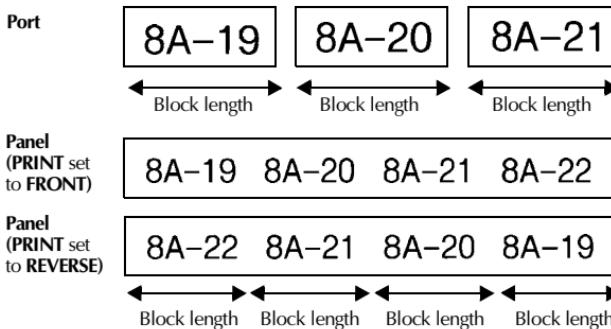
After selecting the **PORT** or **PANEL** Label Type mode, specify the length of each text block or label, and select a frame style if desired. For the **PANEL** Label Type mode, select whether the text blocks are printed in the order that they were typed in or in the reverse order.
