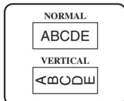
After selecting the Label Type mode **NORMAL** or **VERTICAL**, the label text can be entered, formatted, printed and cut as usual. With the **Normal** Label Type mode, the entered text is printed horizontally along the label. With the **Vertical** Label Type mode, the entered text is printed vertically along the label.
