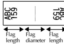
After selecting the **FLAG** Label Type mode, specify the length and diameter of the flag, a frame style if desired, and whether or not to rotate the text.
