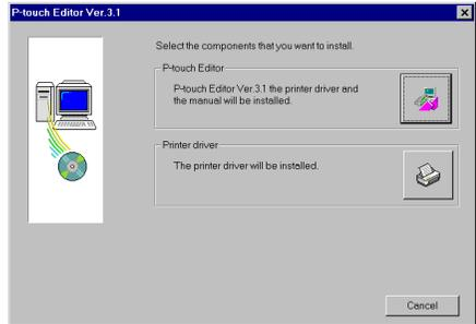
3 Click the bottom button (Printer driver). A Driver Setup dialog box appears, allowing you to select whether to replace, add or delete the PT-2300/2310 printer driver.
