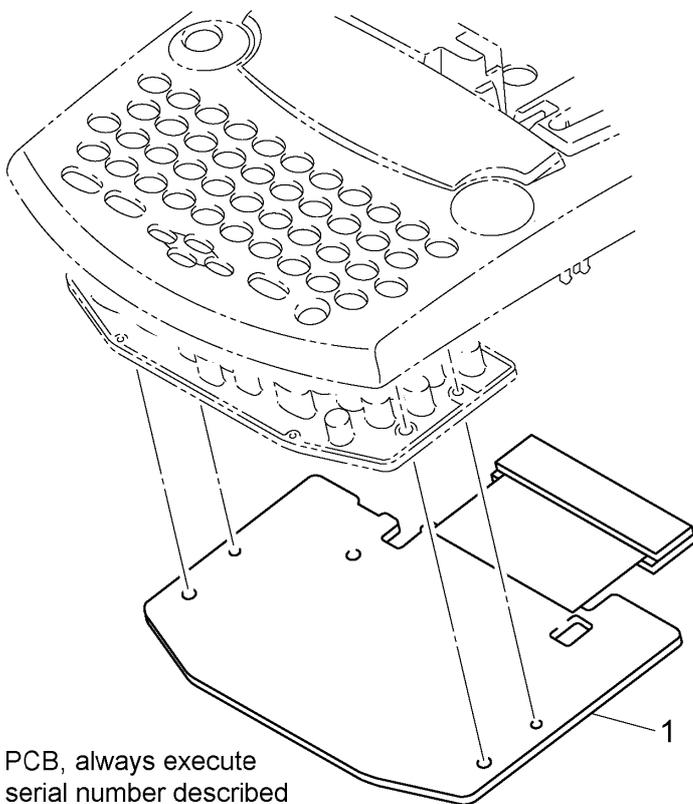
\* After replacing the main PCB, always execute the software to write the serial number described in APPENDICES 1.
